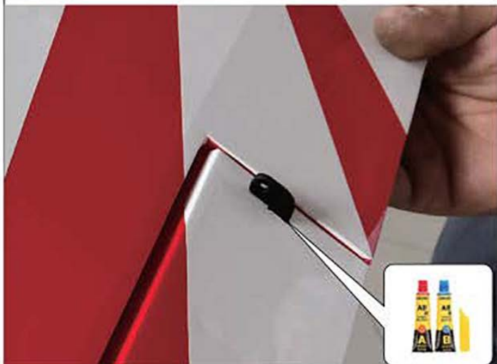
Lower wing aileron control horn installation. Please take note of the horn orientation when installed and see the close up picture below for reference.
