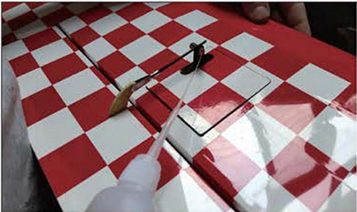
Thread the servo lead through the rib's opening
