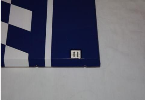
21. Mix a generous batch of epoxy and completely fill the two slots as well as the areas on the control horns and base plates that will glue into both sides of the rudder.
