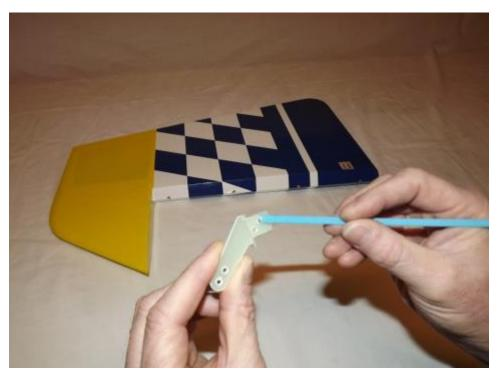
22. Install the rudder horns and base plates into the rudder one side at a time. Clean any excess epoxy from the rudder, recheck the alignment and set the assembly aside to dry. <u>Remember to only install the right side horn if using push-pull!</u>
