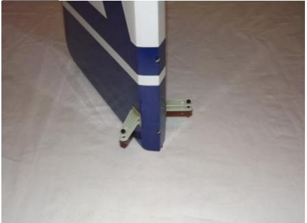
23. Locate the 2mm ball link from the tailwheel hardware bag. There is a predrilled hole to accept the shaft of the ball link. Scuff the shaft of the ball link and glue it into the hole with epoxy as shown below.
