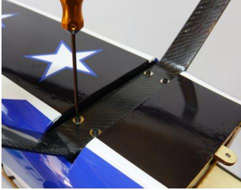
**32.** Trail fit the landing gear fairings and when satisfied with fit secure with Goop style silicon glue. Tape in position until dry.
