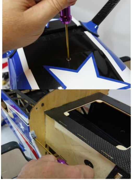
46. Secure the top portion of the cowl to the airframe using 2 3mm bolts inserted through the F1 former and into the blind nuts in the cowl ring.
