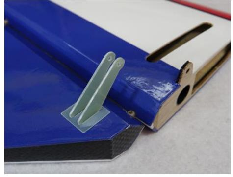
2. Trace around the base plate with a felt tipped marker.
