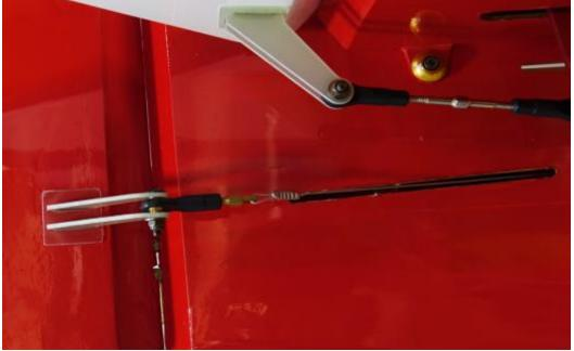
**30.** Here is a photo of the alternate push-pull assembly using the supplied hardware and an EF 1.5" servo arm.
