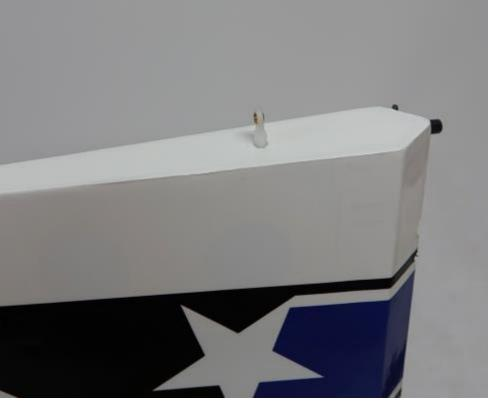
24. Next install the rudder hinges using the same procedure as with the Ailerons and Elevators. Use painters tape to hold the rudder in place while the epoxy dries.
