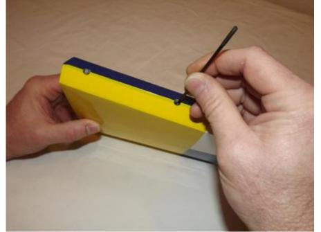
10. Next, coat one side of the hinges with epoxy and push the hinges into the holes of the horizontal stab.
