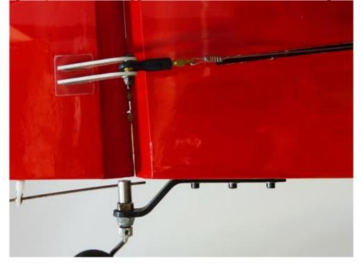
If using the push-pull system use the lower horn location as in this photo
