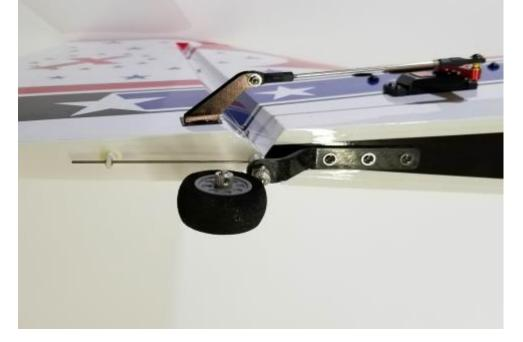
27. If using the pull-pull setup now is the time to install the pull-pull rudder cables. Install the cable onto the brass threaded connector as shown, using the aluminum crimp tube to secure.
