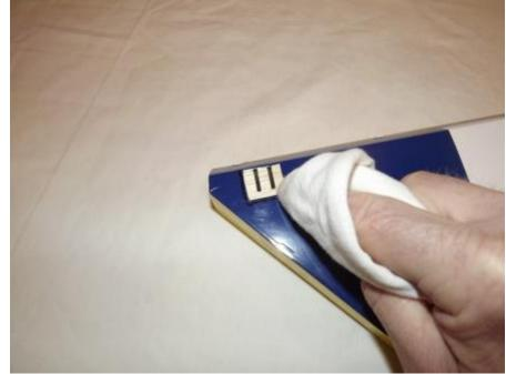
5. Use sandpaper to scuff the portion of the horns and base plate that will be inserted into the elevator.
