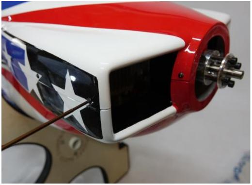
48. Attach a 36 inch EF 20 awg servo extensions to each elevator servo lead. If you plan to remove the stabs for transport, you will need to use 48 inch extensions. Secure with EF Servo Safety Clips or heat shrink tubing. Slide the stab halves onto the carbon fiber stab tube and secure with a 3mm bolt and washer inserted through the mounting tabs and into the pre-mounted blind nuts. Make sure to use a drop of blue Loctite on these bolts.
