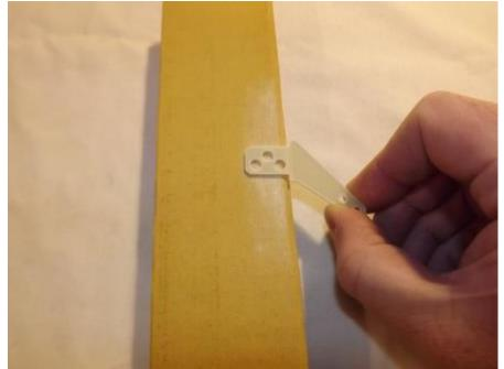
6. Apply 30 minute epoxy to the elevator slots using a zip tie to ensure the slots are filled will epoxy.
