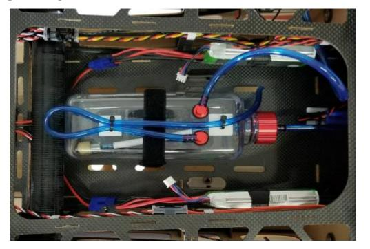
43. Install your switches, batteries and receiver. There are suggested switch mounting locations laser scribed in the fuselage sides visible from the interior of the fuselage. Since switch sizes vary, use a template to ensure you cut the proper size hole for your specific switch. Also, carefully choose the locations to mount your batteries to help achieve correct center of gravity.
