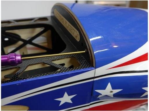
47. Add the remaining bolts to secure the top of the cowl to the lower portion. Use blue Loctite on all bolts!
