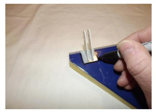
3. Remove the horn assembly and use a #11 blade to remove the covering from inside the ink line you traced around the control horn base.
