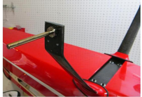
34. Install one wheel collar on the axel first in order to center the wheel in the wheel pant. Next, slide the wheel onto the axel and secure the wheel with the second wheel collar. Repeat this process for the remaining wheel.
