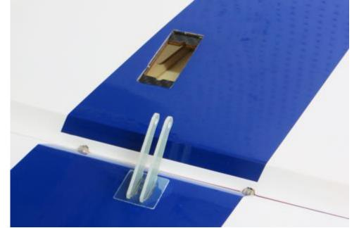
17. Attach a 12 inch EF 20 awg servo extension and secure with a servo safety clip or heat shrink tubing. Install the aileron servo using the manufacturer provided hardware with the output shaft oriented toward the trailing edge of the wing. Electronically center your servo and install the 1.5" EF servo arm and linkage as shown.
