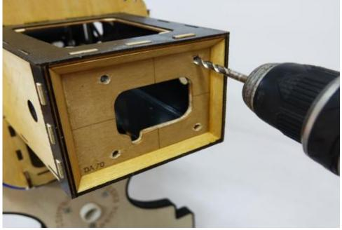
37. If using the DA-70 we highly recommend using our Blazing Star mount for proper engine spacing and cowl-to-spinner clearance. You may find that you need to use the 2mm Delrin spacer for proper clearance. The distance from the motorbox face to the spinner backplate is 6 5/8". If using the spacer be sure it goes between the mount and plywood motorbox face. Mount the engine using 1/4-20x1.75" socket head cap bolts, washers and nylon insert locking nuts.
