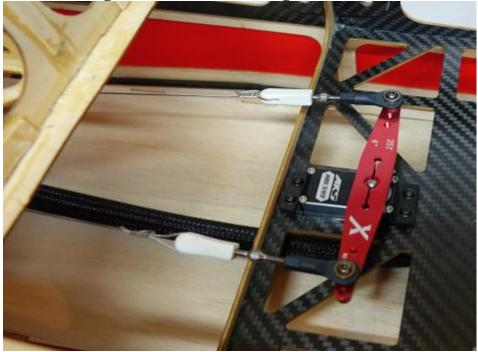
29. This picture shows the exit location of the pull-pull cables as well as the attachment to the rudder horns.
