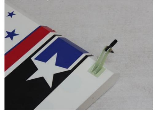
20. Trace around the baseplate with a fine tipped felt marker. Use a sharp #11 blade to remove the covering in this area for the best bond. <u>If using the push-pull system with the rear mounted servo you will only need to glue in the horn assembly on the right side of the rudder (pilot's perspective)</u>. If using pull-pull you will need to use both horn sets.
