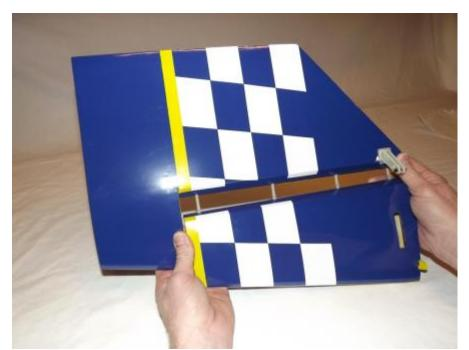
13. Use denatured alcohol and a cloth to remove all excess epoxy, especially on the hinge pin. Make sure you have full deflection in both directions – once satisfied with the results, set the surface aside to dry. After the hinges have dried thoroughly, pull on the surfaces to make sure they are properly secured.
