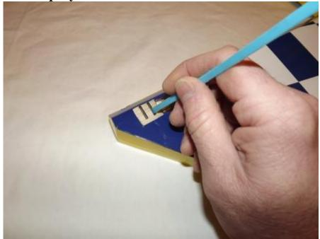
7. Apply a generous amount of epoxy to the bottom of the G-10 control horns and base plate.
