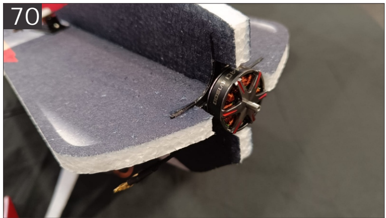
70. Enlarge the pre cut holes over the mount according to need and install the motor on it.
