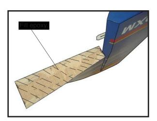
2) While holding the vertical stabilizer firmly in place, use a pen and draw a line on each side of the vertical stabilizer where it meets the top of the fuselage.
