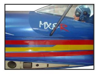
5) Install the canopy and secure it with M2x6mm screws.
