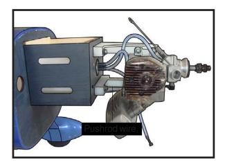
8) Reinstall the servo horn by sliding the connector over the pushrod wire. Center the throttle stick and trim and install the servo horn perpendicular to the servo center line.
