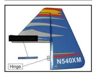
1) Using a modeling knife, remove the covering from over the precut hinge slot cut into the lower rear portion of the tail at the fuselage.
