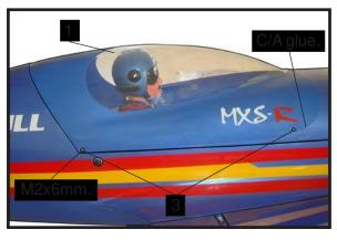
6) Install plastic parts on the fuselage as below picture.
