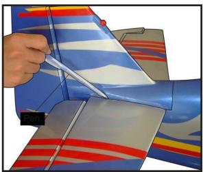
☐ 7) Remove the stabilizer. Using the lines you just drew as a guide, carefully remove the covering from between them using a modeling knife.
