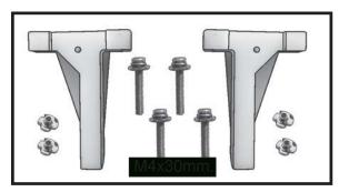
2) Use four M4x30mm head bolts and four 4mm washers to attach the engine mount rails to the firewall. Tighten the screws . Make sure to use threadlock on the screws to help prevent them from vibrating loose.
