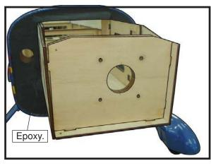
3) Attach the motor to the front of the electric motor box using four 4mm blind nut, four M4x15mm hex head bolts to secure the motor. Please see picture shown.
