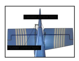
□ 1) Elevator and rudder pushrods assembly follow pictures below.
