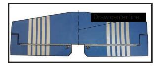
☐ 2) Using a modeling knife, carefully remove the covering at mounting slot of horizontal stabilizer.
