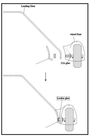
☐ 7) Tighten the setcrews using a hex wrench to secure the collars on the axle over the flat spot to retain the wheel as shown.
