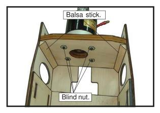
4) Locate the plywood battery tray to the fuselage. Tighten the screws using machine screws M3x15mm to secure the tray in position.
