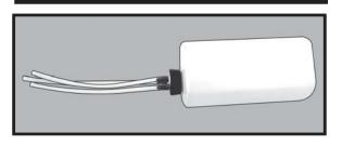
You should mark which tube is the vent and which is the fuel pickup when you attach fuel tubing to the tubes in the stopper. Once the tank is installed inside the fuselage, it may be difficult to determine which is which.
