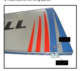
☐ 3) Slide the aileron on the wing panel until there is only a slight gap. The hinge is now centered on the wing panel and aileron. Remove the T-pins and snug the aileron against the wing panel. A gap of 1/64" or less should be maintained between the wing panel and aileron.
