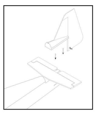
3) Slide the vertical stabilizer back in place. Using a triangle, check to ensure that the vertical stabilizer is aligned 90° to the horizontal stabilizer.
