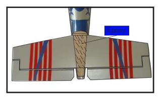
☐ 10) After the epoxy has fully cured, remove the masking tape or T-pins used to hold the stabilizer in place. Carefully inspect the glue joints. Use more epoxy to fill in any gaps that may exist that were not filled previously and clean up the excess using a paper towel and rubbing alcohol.
