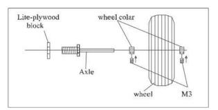
☐ 6) Slide the threaded end of the axle through the hole in the bottom of the landing gear leg. Use a washer and locknut to tighten the axle to the landing gear. Make sure to use threadlock on the nut so it won't vibrate loose in flight as shown.
