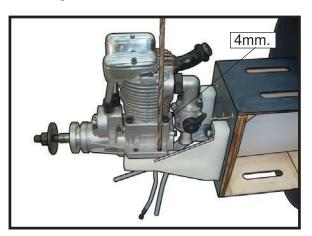
3) Use a drill to drill the four holes in the engine mount rails.
