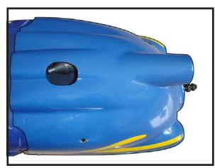
☐ 3) Install the muffler and muffler extension onto the engine and make the cutout in the cowl for muffler clearance. Connect the fuel and pressure lines to the carburetor, muffler and fuel filler valve. Secure the cowl to fuse-lage using the 3x10mm screws.
