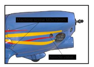
☐ 3) Install the muffler and muffler extension onto the engine and make the cutout in the cowl for muffler clearance. Connect the fuel and pressure lines to the carburetor, muffler and fuel filler valve. Secure the cowl to fuse-lage using the 3x10mm screws.
