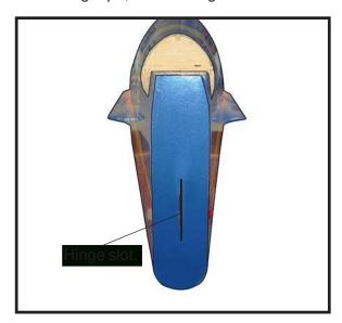
☐ 6) With the stabilizer held firmly in place, use a pen and draw lines onto the stabilizer where it and the fuselage sides meet. Do this on both the right and left sides and top and bottom of the stabilizer.
