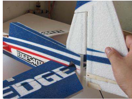
10. Glue the vertical tail with CA.
