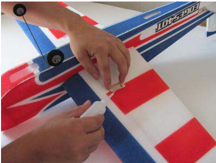
13. Glue the servo frame to the wing. Do this on both sides. Easy on using CA here.
