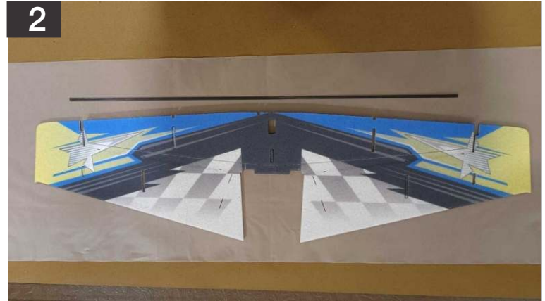
2. Locate the 5mm X 675mm CF Spar shown in the picture above.
