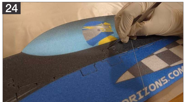
24. We can now begin the vertical fuselage installation, use the blade to separate both the parts.
