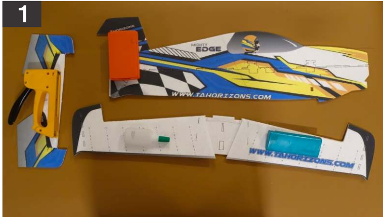
1. (This is mandatory step) locate the hinged items as shown above, Bend them back on to each other as shown and let set for at least 2 hours. This will help to loosen up the movement of the surface.
