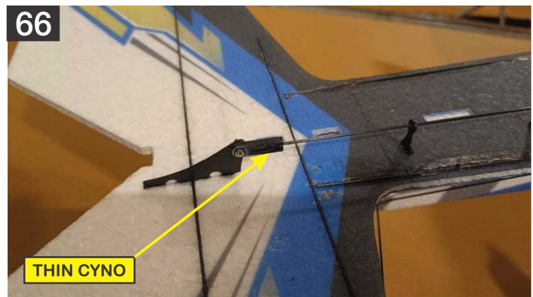
66. Notice how the elevator rod (380mm) is slid in the pre glued pushrod guides, Glue the Elevator control rod on the one side, using thin CA or optionally HV CA.
