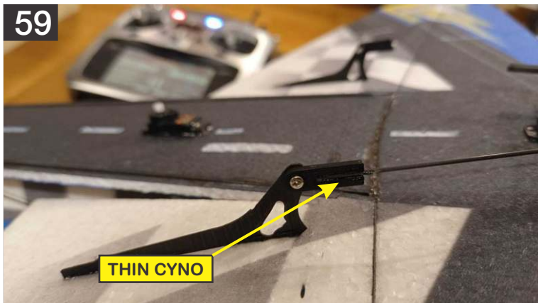
59. Locate the 100mm aileron control rod, glue it on the one side, using thin CA or optionally HV CA. Make sure you have servo arm centered.
