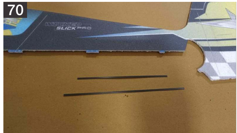
70. Before glueing the upper half of the fuselage, locate the 0.5X3mm (150mmL) stripe and 0.5X3mm (200mmL) stripe. these will be used to strengthen the vertical tail and rudder section.
