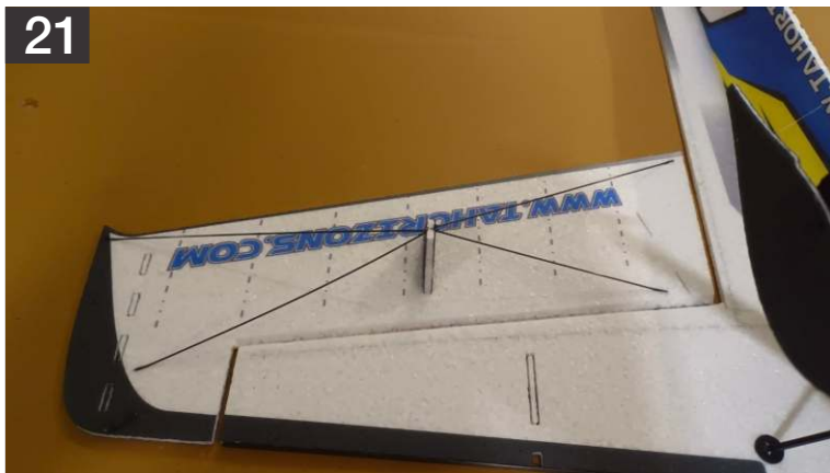
21. Locate the triangular joiner that will be placed on the underside of each aileron. Once you make sure that it fits clean and snug into the cutout, you can glue this piece in and repeat to the other side.
