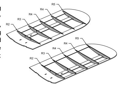
11 Fit WS1 and WS2 into the slots in R1.
