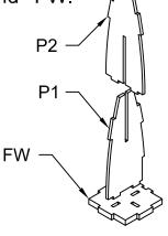
2. Secure the motor mount to the firewall FW. Use the etched lines for proper motor mount alignment.
