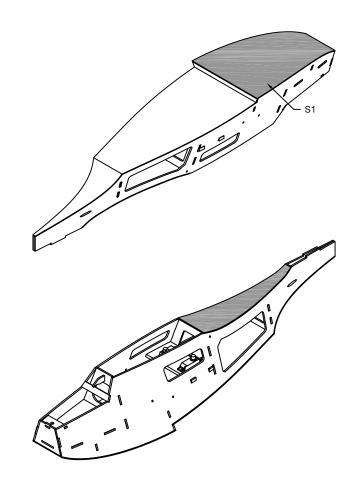
34. Sand the fuselage sides flush with the face of former F1. Stack and glue the  $\frac{1}{4}$ " balsa nose blocks to F1. Glue S5 in place.
