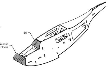
35. Sand the fuselage sides. Check the fit of the battery hatch, sand as necessary for a good fit.
