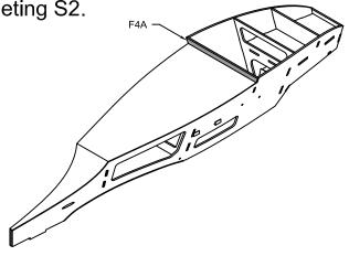
32. Sand F4A flush with the bottom of the fuselage. Glue sheeting S1 to the bottom of the fuselage.
