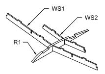
12. Fit and glue the wing spar assembly into the slots in R2, R3 and the wing panel. Do not glue R1 to the wing panel yet.
