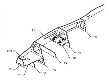
27. Fit fuselage side FL to formers F1-F6, Battery Tray (BT) and servo tray (ST). Ensure all parts are fully seated into their slots and glue together in the following order:
