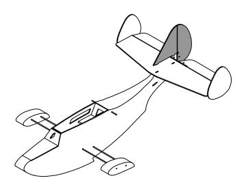
41. Glue the vertical stabilizer sub fin to the bottom of the fuselage.
