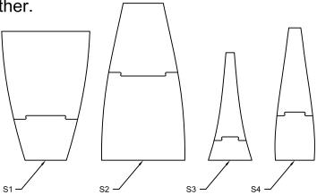
**30.** Use a sanding bar to sand the bottom of the fuselage sides and formers. Glue sheeting S3 to the fuselage bottom first, allow sheeting to overlap all edges.
