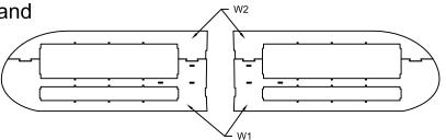
10. Fit and glue ribs R2-R5 to the wing panels. It is recommended to start by gluing the ribs to the trailing edge first, then the center and finally the leading edge. Make sure the ribs are fully seated into the notches in the trailing edge before gluing in place. Be sure to build a right and left wing panel.
