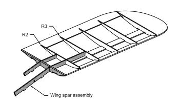
13. Fit and glue the second wing panel and wing spar assembly together. Make sure the leading and trailing edges of both wing panels are aligned and glue R1 to both wing panels.
