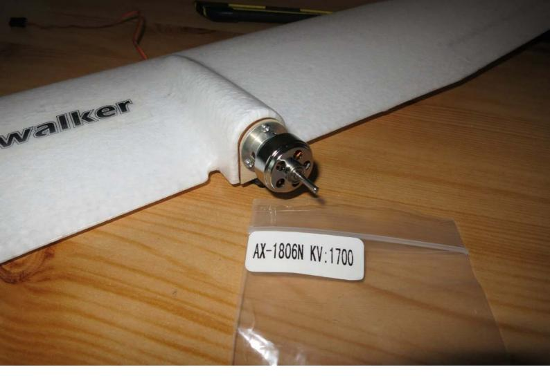
Mini skywalker is suitable for AX1806N motor
