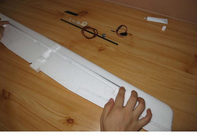
First we stick wing's carbon-fiber bracing sheet, evenly daub glue after waiting for 3 minutes, then press in formation.
