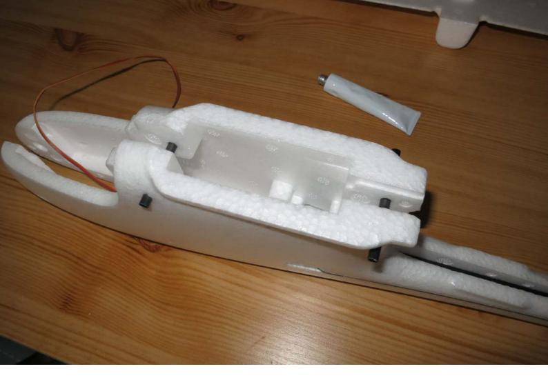
Spread the glue evenly on both sides of the fuselage and wait for 5 minutes, then stick, pay attention to the glue layer thickness cannot be too much.
