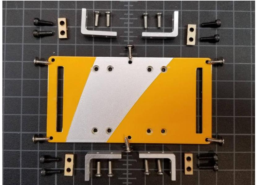
Begin by attaching the aluminum servo brackets to the wing panel. Mark the panel with an arrow indicating the aircraft forward direction. This helps you keep the mounting orientation straight.
