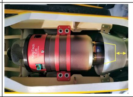
Check both horizontal and vertical alignment of the turbine and exhaust pipe. When looking in from the rear of the exhaust pipe, you should see that the turbine is centered.
