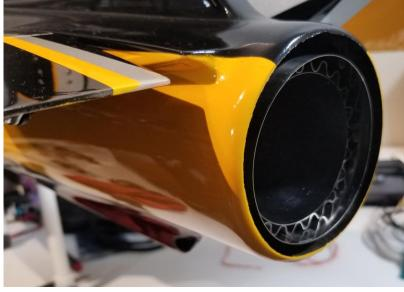
Place the turbine on the plywood mounts as shown. Your arrangement may differ slightly depending on the turbine you're using. The turbine exhaust should sit within the exhaust pipe bell and be within 25mm of the beginning of the exhaust pipe as illustrated here.
