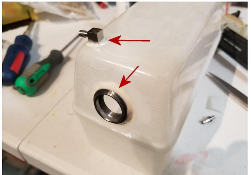
Install the fittings you need onto the fuel tank cap. Depending on your needs, you may want to use different fittings. Use a small amount of Hysol epoxy on the fitting threads to seal and secure them.
