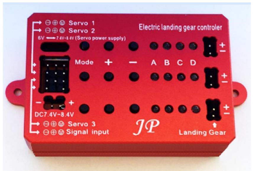
Each landing gear unit can operate in one of two modes as show here. For this build, we are only worried about configuring Mode 1 for the nose gear door sequencing. We will use the “Servo 1” port for our nose gear door servo.
