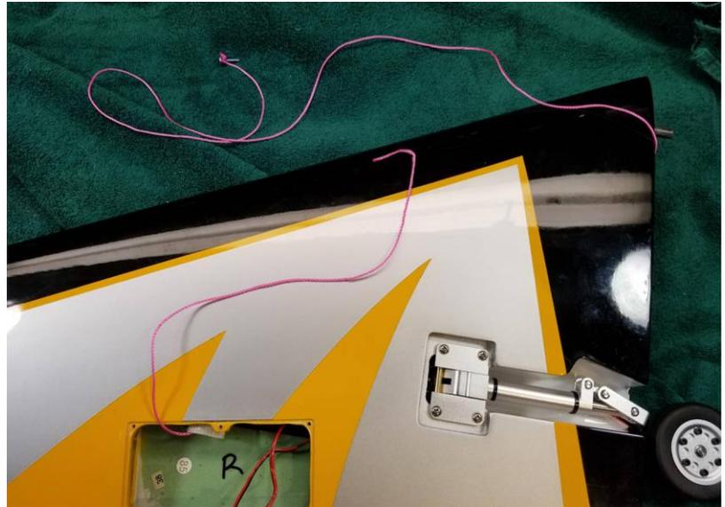
From the servo area, drop the screw through the fiberglass tube toward the leading edge of the wing. Tilt the wing up to drop the screw with the string down to the root of the wing.
