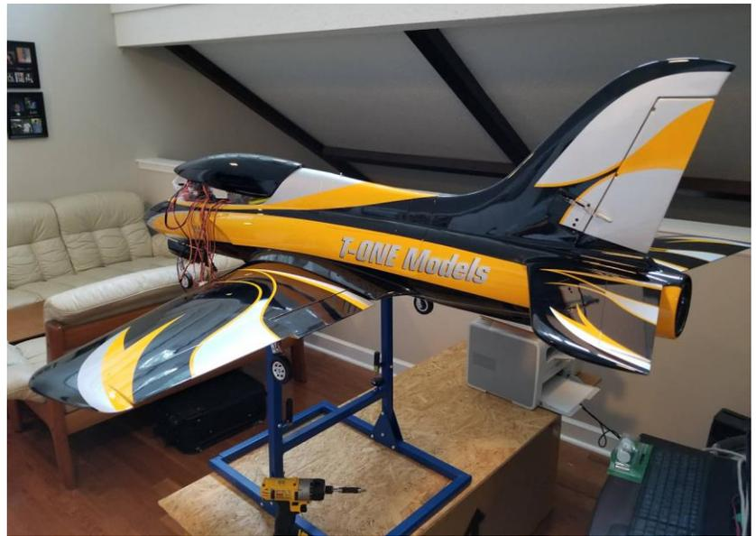
This section of the build will vary drastically from aircraft to aircraft depending on the equipment being used. Use whatever layout suites your needs best. In the layout shown here, the main gear controller is under the deck and the radio and turbine batteries are to the left on the deck above the nose gear. The fuel ball valve holder is my own design and can be downloaded and printed from [Thingiverse](#).
