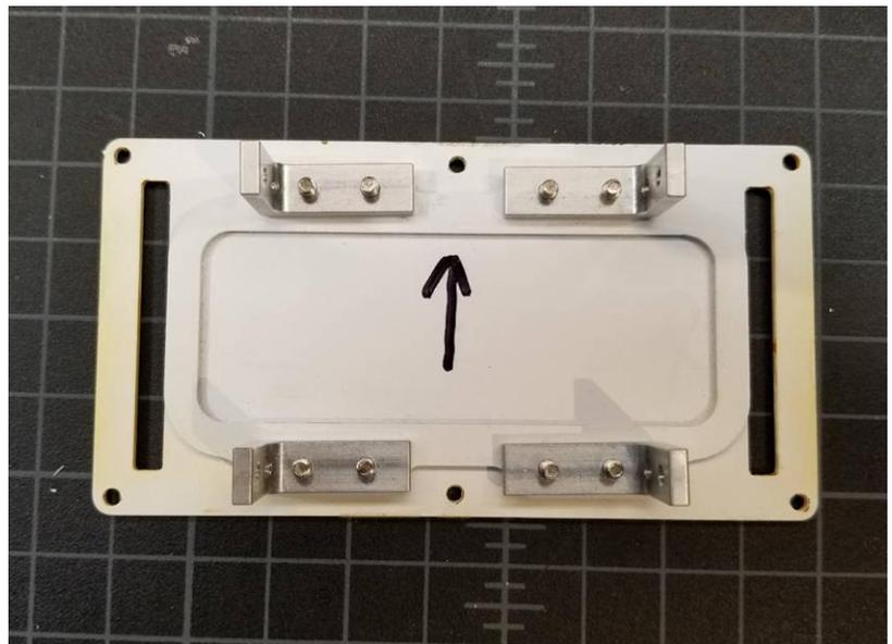
There are plenty of spacers included in the kit to achieve the proper spacing of the servo arm within the slot in the wing panel. You want to mount the servo so that the arm protrudes directly in the middle of the slot.
