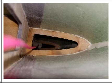
This is the wing section of wiring harness. Due to the different lengths of servo, gear, and brake wires and their corresponding connections on the harness, you'll be pulling back and forth a few times.
