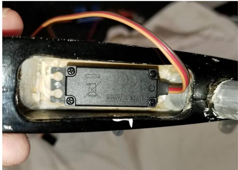
Using the Savox SV1250MG servos in this build, the servo did not sit deep-enough in its mount for the arm to be in the middle of the slot as shown.
