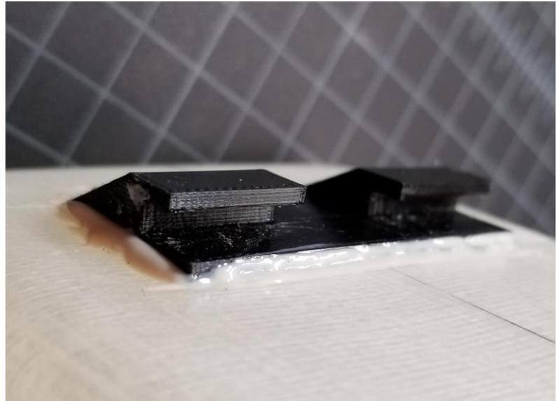
This is the bracket for the bottom front of the tank. Two M3 self-tapping screws are used to hold the tank in place. In addition to securing the front of the tank, this bracket holds the tank forward so the bottom rear bracket stays firmly seated under the plywood deck. These parts are available for downloading and printing here: <https://www.thingiverse.com/thing:3124330>
