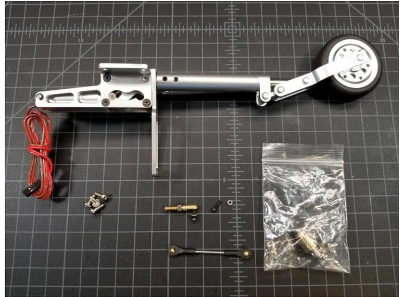
Mount the nose steering servo in the configuration shown.
