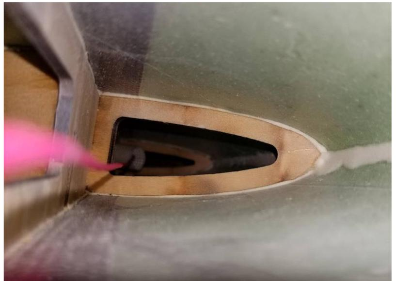
This is the wing section of wiring harness. Due to the different lengths of servo, gear, and brake wires and their corresponding connections on the harness, you'll be pulling back and forth a few times.
