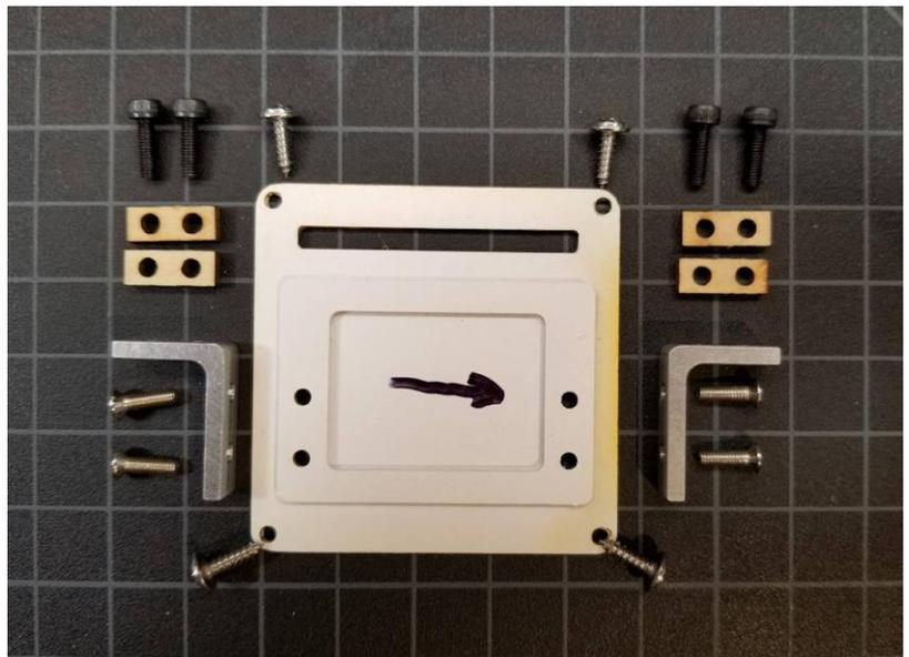
Assemble the rudder servo mounting as shown. I needed to use two of the wood spacers that came with the kit. I happen to have some aluminum spacers that fit perfectly. Ensure the servo arm protrudes in the center of the slot and there is no rubbing or binding with the arm.
