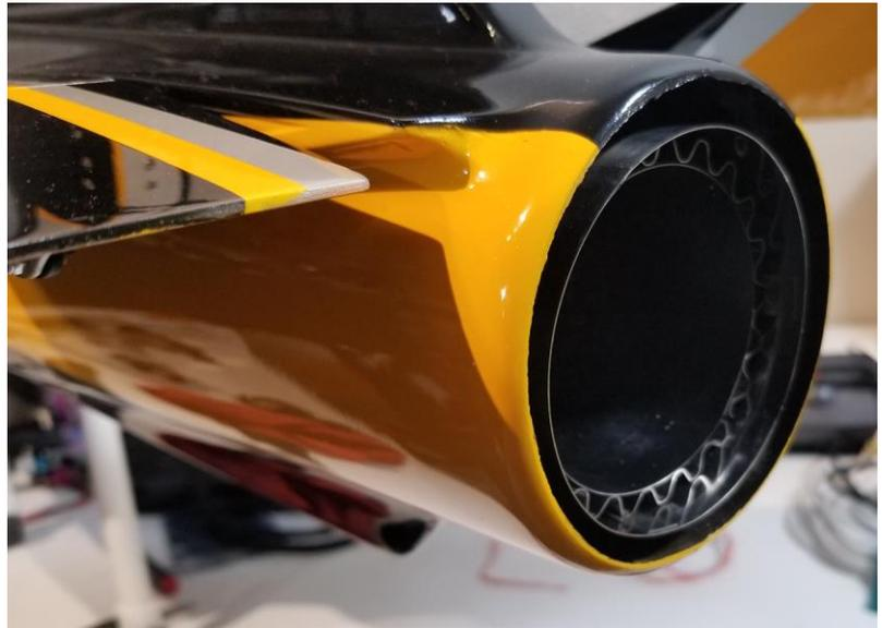
Place the turbine on the plywood mounts as shown. Your arrangement may differ slightly depending on the turbine you're using. The turbine exhaust should sit within the exhaust pipe bell and be within 25mm of the beginning of the exhaust pipe as illustrated here.
