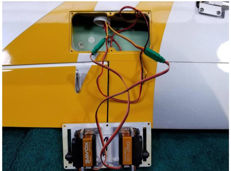
When you're done, you should have the harness coming out of the wing as shown here. You should have enough slack to have the wing pulled away from the body to retract the gear during disassembly.
