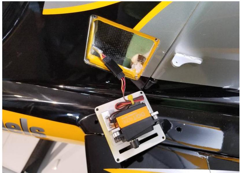
Install the rudder linkage as shown. The control surface horn aligns with the servo arm so a two-clevis setup was used. Use your preferred method to secure the clevis' such as fuel tubing as shown.
