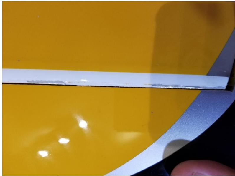
This is easily resolved by using a common emery board to gently smooth the underside/inside the flight surface and the top/outside on the control surface. Go slow and don't be too aggressive with the file to avoid removing too much material.
