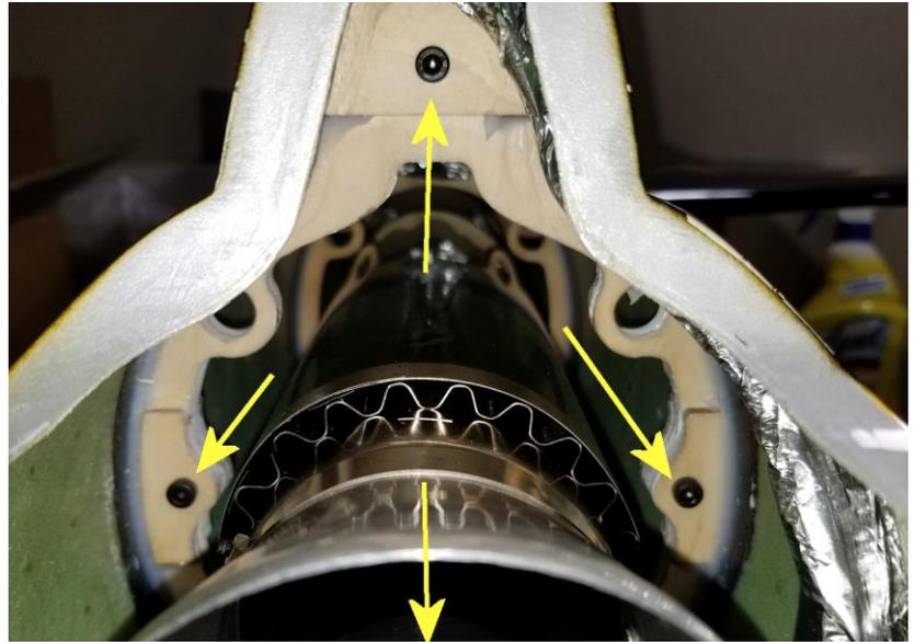
Ensure proper alignment of the tail section with the main fuse before the final tightening of the bolts.
