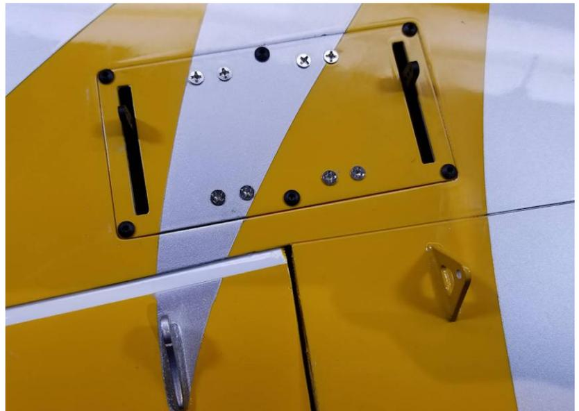
This is the layout of wing servo linkage hardware.
