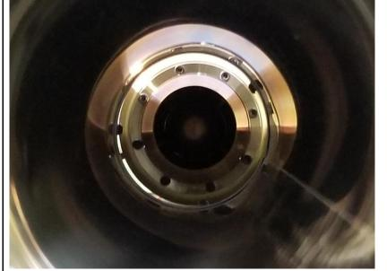
Once you are confident with the placement and alignment of the turbine and pipe. Mark the holes for mounting and predrill. Use selftapping or wood screws to complete the installation.
