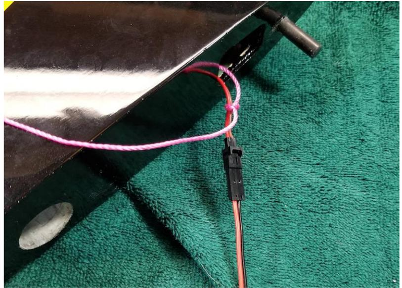
Find the appropriate wing servo assembly you set aside earlier and make the appropriate connections. Make sure you secure these connections using your preferred method such as a servo plug bracket or heat shrink tubing.
