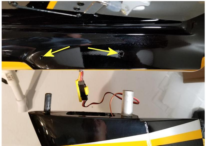
Ensure there is no binding of the moving control surface against the airframe.
