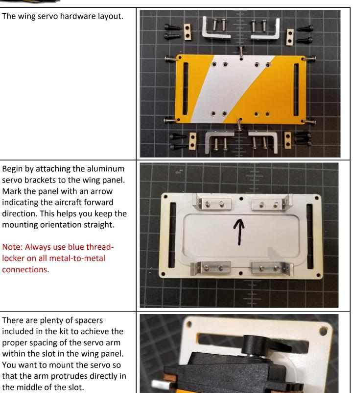
The servos should be mounted with the arms closest to the front of the aircraft.
