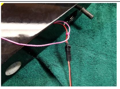
Find the appropriate wing servo assembly you set aside earlier and make the appropriate connections. Make sure you secure these connections using your preferred method such as a servo plug bracket or heat shrink tubing.
