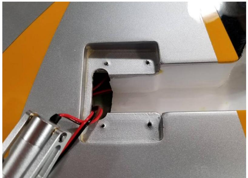
Mount the main gear and feed the gear and brake wires to the wing servo access area as shown.
