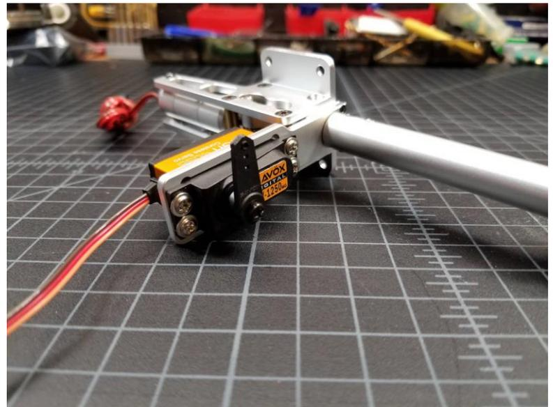
Install the nose gear steering horn and its locking nut as shown. Tighten the brass arm to the orientation pictured then tighten the locking nut against the gear shaft to hold in place.
