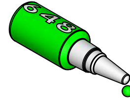
Use Loctite 648 Bonding
