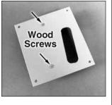
□ □ 4. Glue the blocks to the servo cover. Once the glue has cured, drill a 1/16" [1.6mm] hole through the cover and into the servo mounting blocks. Secure the block to the cover with a  $#2 \times 3/8"$  [ $#2 \times 9.5$ mm] wood screw. Do this for both of the servo covers.
