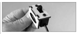
□ 39. Mount the switch using just the screws that came with the switch. Glue the switch mount to the fuselage as shown in the picture in the next step.
