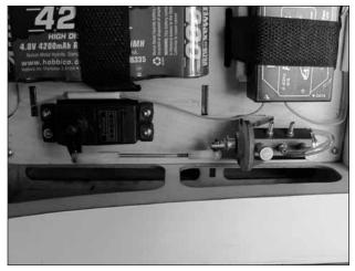
□ 30. Thread a nylon ball link onto one of the .074 × 6" [152mm] wires threaded on one end. Snap the ball link onto the ball on the air control valve. Center the servo and the air control valve. Make a mark on the wire when it is aligned with the outer hole in the servo arm. Make a 90 degree bend on the mark. Cut off the excess wire 3/8" [9.5mm] above the bend. Insert the wire into the outer hole of the servo arm. Install a Faslink<sup>™</sup> onto the wire to secure it to the servo.
