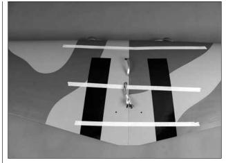
□ 4. When you are satisfied with the fit of the joiner, glue the joiner into the wing joiner pockets with 30-minute epoxy. When gluing the wings together be sure that you use plenty of glue in the joiner pockets, the joiner and the root ribs of the wing. Use masking tape to hold the wings together while the glue cures.
