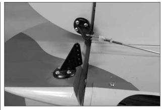
☐ 4. Mount the control horns to the elevators and the rudder. Follow the same procedure used for the ailerons, by drilling 3/32" [2.4mm] holes and using #4 × 1/2" [12.7mm] sheet metal screws. Attach the elevator clevis in the third hole from base of the control horn. Don't forget to harden the holes with thin CA after first installing, then removing the screws.
