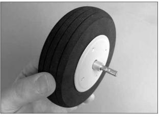
$\Box$   $\Box$  16. Slide the axle into the wheel from the side without the wheel cover; then, slide the aluminum tube over the axle.
