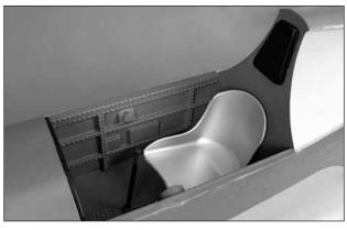
□ 3. Glue the cockpit floor into the fuselage followed by the two side walls. When the glue has dried glue the seat to the pedestal molded into the cockpit floor.
