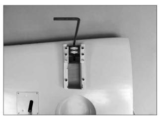
□ □ 7. Insert the **landing gear wire** into the hole in the landing gear block. The axle of the wire must be
