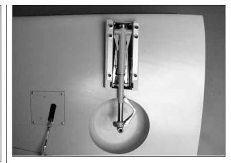
□ □ 3. Install the right side **landing gear** between the mounting blocks. The landing gear fits between the blocks best if you install it with the gear retracted. Mount the landing gear and the blocks with six 8-32 × 2-1/2 [64mm] socket head cap screws, #8 flat washers and #8 lock washers.
