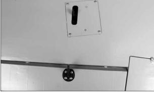
□ □ 10. Place a black nylon control horn onto the plywood mounting plate in the aileron in line with the servo arm. Drill a 3/32" [2.4mm] hole through each of the holes in the control horn. Drill only through the plywood plate. Do not drill through the top of the control surface. Mount the horn with four #4 × 3/8" screws.
