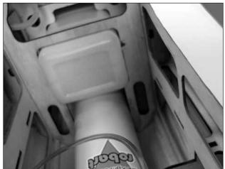
□ 11. Install the fuel tank into the opening in the fuselage as shown. Feed the lines through the fuselage up to the firewall. Make sure when you insert the tank that the vent line is at the top of the tank.
