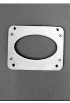
□ 2. We have included 1/8" [3.2mm] plywood spacers to help space different engines out the required distance for the engine to fit the cowl. Drill a 3/16" [4.8mm] hole through the "+" marks on one of the plywood spacers. It's a good idea to fuel proof the spacer. This can be done by brushing a coat of 6-minute epoxy thinned with alcohol, or a coat of paint.
