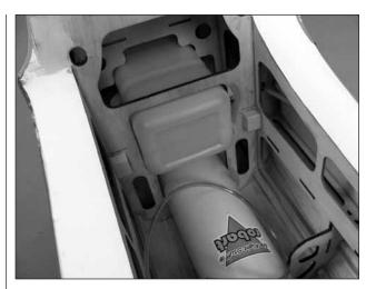
□ 24. 1/8" [3.2mm] below the marks you made make another line. Glue a 3/8" × 1/2" × 5/8" [9.5mm × 13mm 16mm] hardwood block so that the top of the block is aligned with the new line you just made. The tray will rest on and be screwed into the blocks. Once the glue has cured place the tray onto the blocks. Drill a 1/16" [1.6mm] hole through the holes in the corners of the tray into the blocks and then remove the tray.
