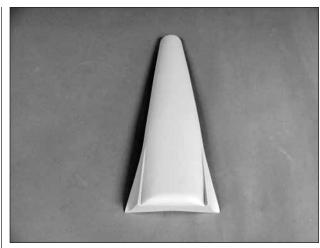
$\Box$  6. Mount the wing to the fuselage with the two 1/4-20 × 2" [51mm] nylon wing bolts. Locate the fiberglass belly pan. Place it on the wing. With a fine-tip felt pen, mark the location on the wing for the belly pan.
