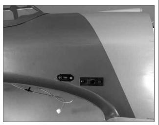
$\Box$  29. Install your radio switch and charge jack in the fuselage. Locate this switch as far away from the ignition switch and battery as is practical. It is generally recommended that you maintain 6"-10"
