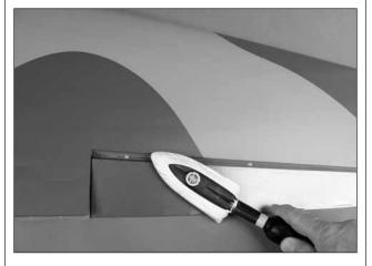
□ 2. Use a covering iron with a covering sock on high heat to tighten the covering if necessary. Do this for all of the components of the model. Apply pressure over sheeted areas to **thoroughly** bond the covering to the wood.
