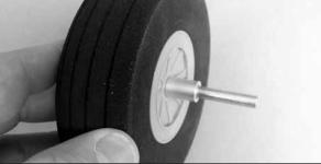
□ □ 11. Locate a wheel, the 5/8" [16mm] long aluminum tube and the axle included with the landing gear. Slide the axle into the wheel and slide the aluminum tube over the axle.
