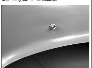
□ 27. Determine where you would like to mount the air fill valve on your fuselage. Make a 5/16" [8mm] hole in the fuselage and then install the valve in the side of the fuselage. Install a "T" fitting in the air line between
