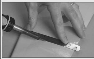
Use a soldering iron to cut the covering from the stab. The tip of the soldering iron doesn't have to be sharp, but a fine tip does work best. Allow the iron to heat fully. Use a straightedge to guide the soldering iron at a rate that will just melt the covering and not burn into the wood. The hotter the soldering iron, the faster it must travel to melt a fine cut. Peel off the covering.
