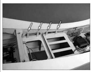
□ 34. Route the air lines from the tailwheel through the fuselage and secure them. We used some scraps of balsa to secure them to the fuselage as shown.
