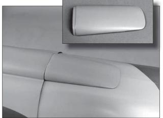
□ 9. Locate the fiberglass cowl extension. Slide it in place under the cowl. Trace the outline of the extension onto the fuselage. Remove the extension. Cut the covering from the fuselage using the same technique described on page 16. Glue the extension in place on the fuselage.
