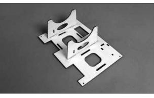
□ 15. Locate the three components of the radio / servo tray. Glue the tray together as shown making sure that you glue the two parts with the arc into the main tray exactly as shown in the photo.
