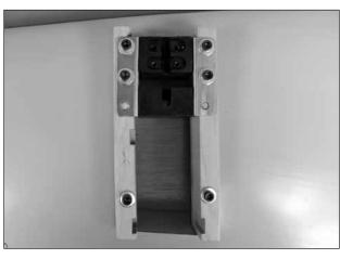
□ □ 5. Double-check both of the landing gear block installations to be sure they are correct. When you are satisfied with the installation remove the bolts from the right wing panel. Mix a 1/2 ounce [4 drams] of 30-minute epoxy. Use an epoxy brush to apply a film of glue to the bottom of the landing gear mounting blocks and to the rails in the wing as well as the sides of the box the mounts slide into. Be careful not to get glue into the blind nuts. If you get glue into the threads of the
