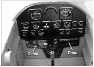
□ 4. Install the two instrument panel decals to the panel. Complete the cockpit by gluing the instrument panel, control stick and headrest in place as shown.
