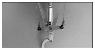
□ 9. Now pull on the long end of the cable to reduce the size of the first loop. Slip the loop over one of the ball link balls on the steering arm. Tighten the loop until it is small enough to remain secure on the ball, yet may still be pried off. Squeeze the swage with pliers. Connect the other cable to the other ball link ball the same way.
