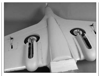
□ 9. Apply epoxy to the belly pan flange. Then glue the belly pan in place on the fuselage. Tape the belly pan in place until the glue cures.
