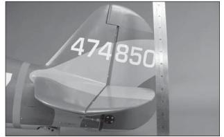
□ 3. Move the elevator up with your transmitter and move the ruler forward so it will remain in contact with the trailing edge. The distance the elevator moves up from center is the "up" elevator throw. Measure the down elevator throw the same way.
