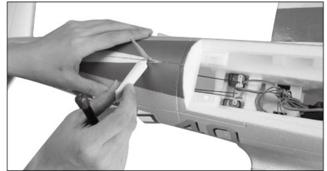
12 Install the scale antenna set with the glue.
