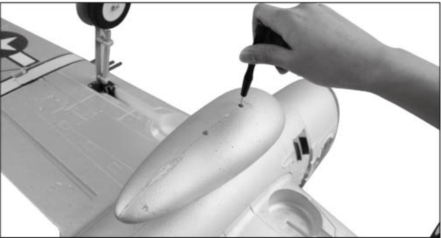
11 Fix the fuel tank with PA2.3x20mm screws.
