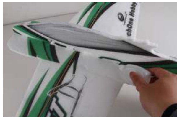
Insert upper fuselage into the slots on horizontal fuselage, then fix with glue.
