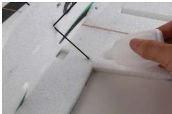
Glue round doublers on pre-reserved holes on wing, then install landing gear as picture shown and fix with glue.
