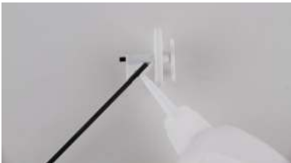
Insert 2×220mm carbon fiber rod into the slot on triangle part, then fix with glue.
