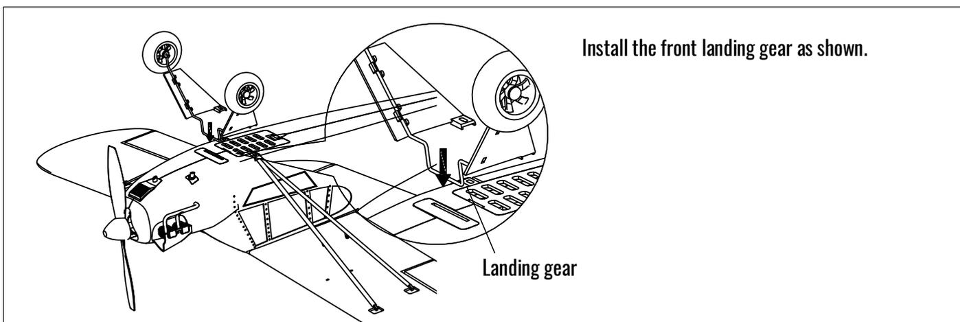
Install the front landing gear as shown.
