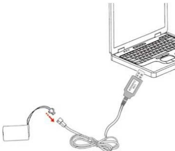
Connect the USB charging cable to a USB socket on a PC, laptop or smartphone charger. Then connect the flight battery to the charging cable.
