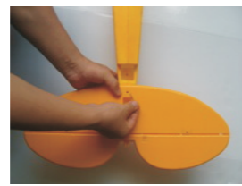
4 Install the horizontal tail in fuselage with screw (PM3.0mmX30mm 2pcs)
