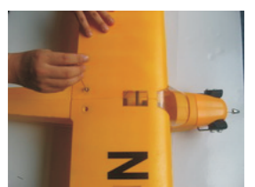
5 Install the main wing and cabin with screws. (PM3.0X35mm 2pcs)
