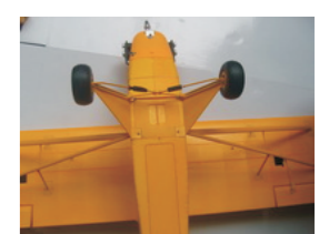
8 Tighten diagonal draw bar and dam-board with screws. (PA2.6X20mm)
