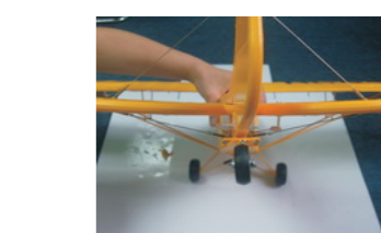
9 Fix the horizontal wing and vertical wing with spring wire (spring :0.5X4X24.1mm 8pcs For horizontal 1.0X94mm 2pcs For vertical 1.0*94mm 2 pcs)
