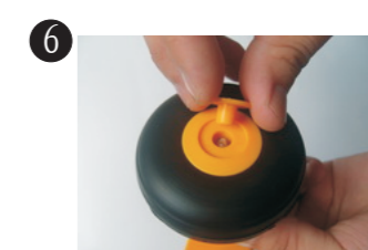
Screw the wheel chock and wheel into the steel wire to ensure the flexible rotation of wheel.
