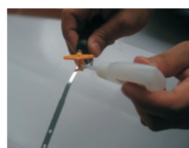
7 Fix the rear landing gear with screw. (PA2.6X8mm 2pcs)
