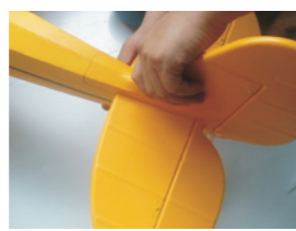
5 Install the vertical tail in fuselage with screw (PM3.0X45mm 1pcs, PM3.0X40mm 1pcs).
