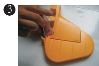
3 Install the screw horns in the steering holder with screw. PA1.7X15mm 2pcs
