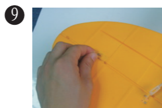
9 Fix the horizontal wing and vertical wing with spring wire (spring :0.5X4X24.1mm 8pcs For horizontal 1.0X94mm 2pcs For vertical 1.0*94mm 2 pcs)
