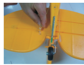
8 Fix one end of the spring in the steering holder, the other end to steering arm, close the chuck after leveling elevator. 0.5X4X24.8mm 2pcs
