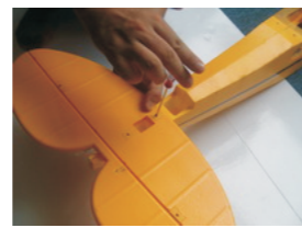
3 Install the screw horns in the steering holder with screw. PA1.7X15mm 2pcs
