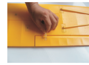
2 Install the steel wire with the second hole on servo arm, close the chuck after leveling aileron. (1.2X65mm 2pcs)
