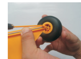
Screw the wheel into the steel wire in clockwise direction.
