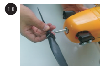
10 Fix propeller into the spindle of motor. Then tighten it up with spacer and screw.
