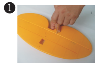
1 Install the screw horns in the horizontal tail. (PA1.7X15mm 4pcs)
