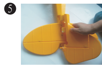
5 Install the vertical tail in fuselage with screw (PM3.0X45mm 1pcs, PM3.0X40mm 1pcs).
