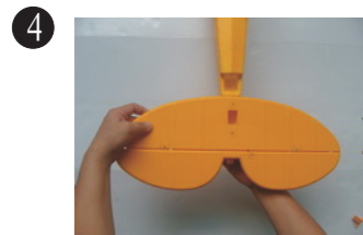
4 Install the horizontal tail in fuselage with screw (PM3.0mmX30mm 2pcs)
