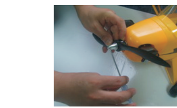
10 Fix propeller into the spindle of motor. Then tighten it up with spacer and screw.
