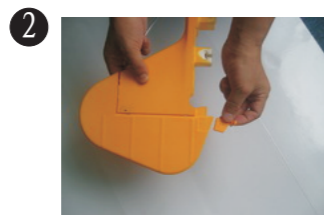
2 Install the steering holder in the vertical tail.
