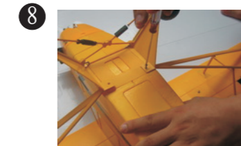
8 Tighten diagonal draw bar and dam-board with screws. (PA2.6X20mm)
