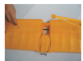
3 Put reinforcing rod into the holes on left and right wing with two ends. Then fasten reinforcing rod with screws.
