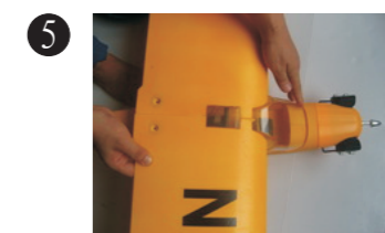
5 Install the main wing and cabin with screws. (PM3.0X35mm 2pcs)
