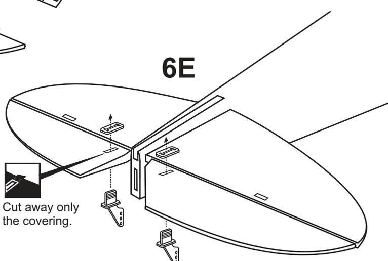
Apply a thin layer of machine oil or petroleum jelly to only the pivot point of the hinges on the elevator, then push the elevator and its hinges into the hinge slots in the trailing edge of the horizontal stabilizer. There should be a minimal hinge gap. When satisfied with the alignment, hinge the elevator to the horizontal stabilizer using CA glue.
