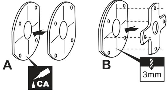
Using a aluminum motor mounting plate as a template, mark the plywood motor mounting plate where the four holes are to be drilled (2).
