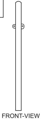
Trial fit the vertical stabilizer in place. Check the alignment of the vertical stabilizer.
