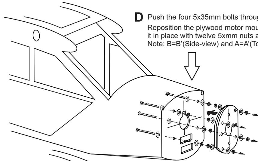
**D** Push the four 5x35mm bolts through the fire-wall as shown (5).
