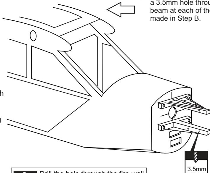
Drill the hole through the fire-wall for the plastic pushrod tube
