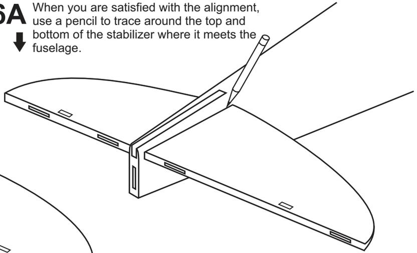
**6B** Remove the horizontal stabilizer from the fuselage. Using the sharp hobby knife, carefully cut away the covering inside the lines which were marked above.
