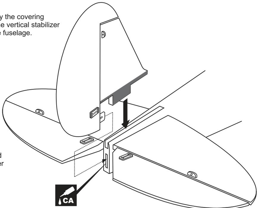
Install the vertical stabilizer into the fuselage and adust the alignment. Secure the vertical stabilizer in place using CA glue.
