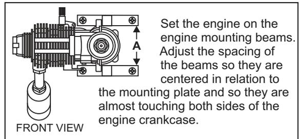
**B** Position the engine on the engine mount beams so the distance from the prop hub to the fire-wall is 102mm/(4"). Using a pencil, mark the engine mounting plate where the four holes are to be drilled. Note: Mark the mounting plate through the engine mounting flanges.
