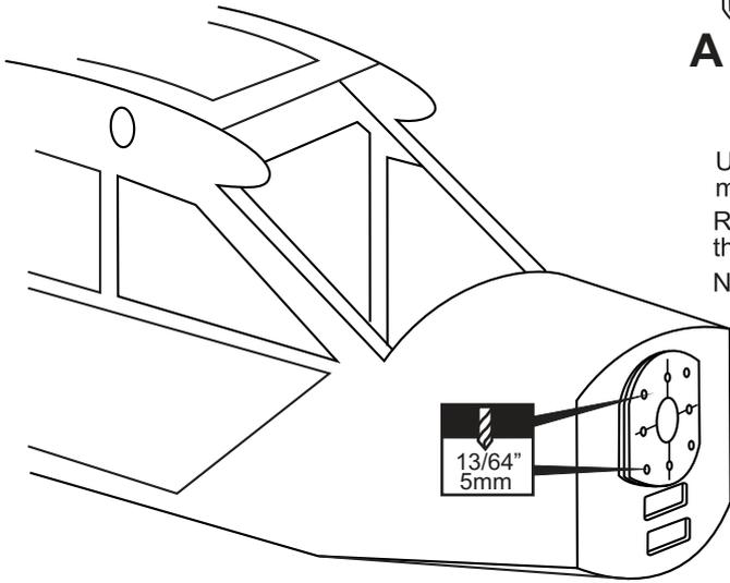
**C** Using a plywood motor mounting plate as a template, mark the fire wall where the four holes are to be drilled .
