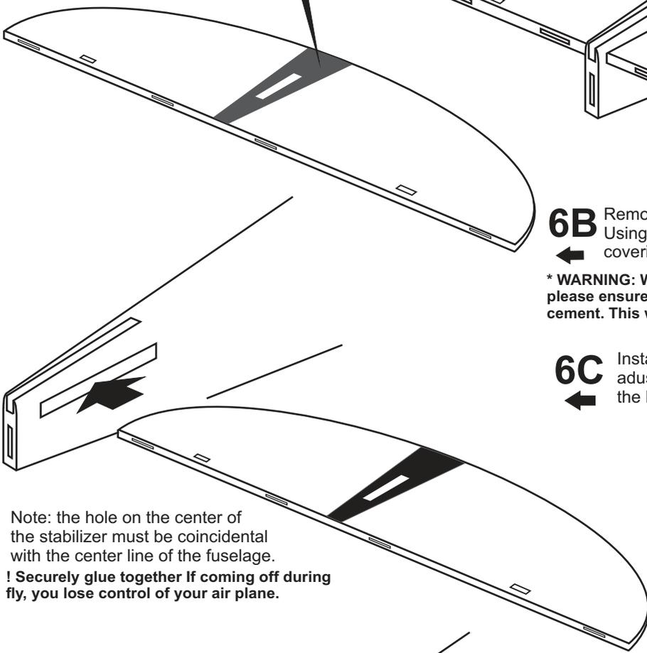
Note: the hole on the center of the stabilizer must be coincidental with the center line of the fuselage.
