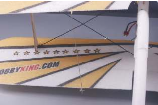
57. Insert the end of the Z wire into the ailerons control horns in the upper wing . Insert the other end of Z wire into the pushrod connectors in the lower wing.
