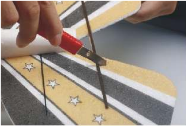
18. Using the sharp knife cut the slots for control horn (elevator).
