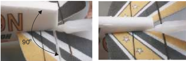
17. The horizontal stabilizer into the fuselage glue around the edge with CA glue. check the perpendicularity as shown.
