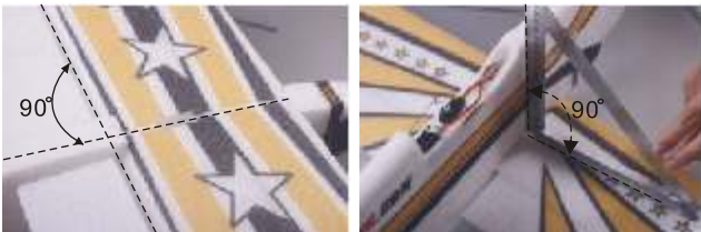
34. Insert wing left and right into the fuselage as shown .check if the wing is in the centre and alignment . Also check if the wings is perpendicular to the fuselage side.
