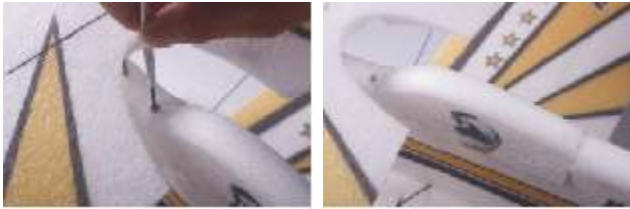
54. Install the canopy to the fuselage with screw and connector
