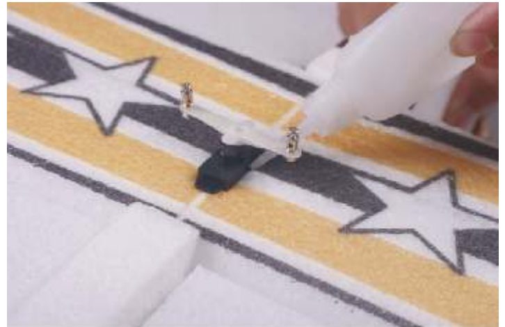
37. Insert the aileron servo into the hole and the servo cable through the opening for receiver. Switch on the RC -SET to have the servo in neutral . Install the servo arm on the servo . Using CA glue .
