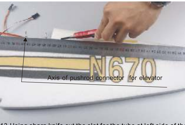
13. Using sharp knife cut the slot for the tube at left side of the fuselage .the slot must Be 3mm deep .position slot as shown.
