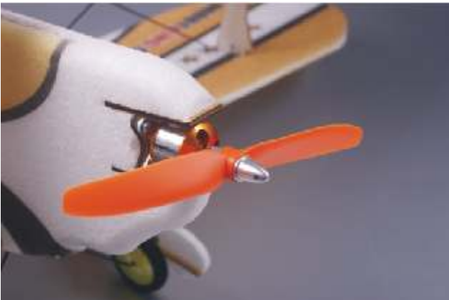
58. Install the the propeller and spinner to the motor .tighten properly.
