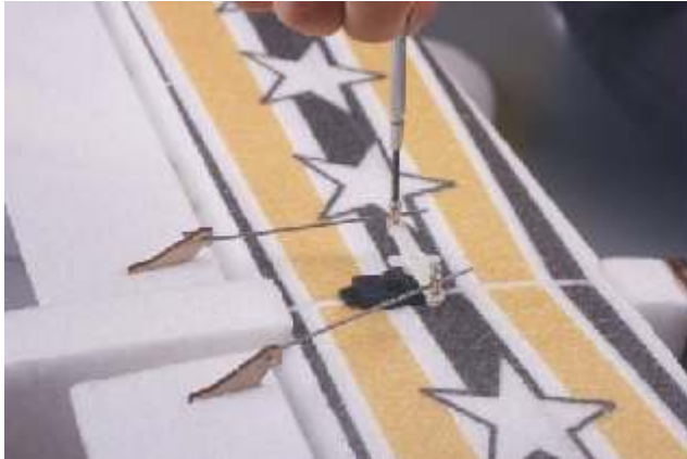
40. Insert the control wire into the ailerons horns and into aileron servo arms as shown . Switch on the rc-system to have the servo in neutral . Put the ailerons in neutral . Now the pushrod connectors screws must be tightened.
