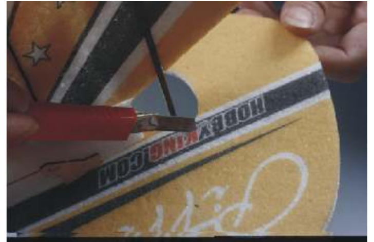
22. Using the sharp knife cut the slots for control horn (rudder).
