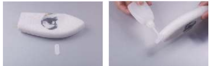
53. Fix the end of PVC without hole to the front of the canopy with glue.
