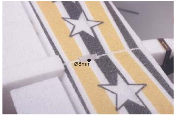
36. Cut a 8mm deep hole on the lower wing for aileron servo.
