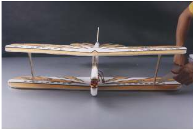
48. Insert the upper wing on the baldachin and the wing struts as shown.
