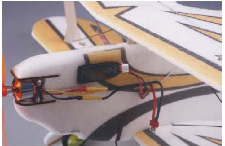
60. The accu pack press into the hole in fuselage .
