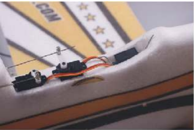
41. Insert the receiver into right place . The fuselage foam will hold it in place . plug the elevator , rudder and aileron servos and ESC connectors into receiver.
