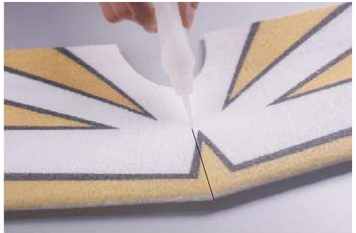
44. On the flat board glue the up wing panels together using CA glue and activator spray.
