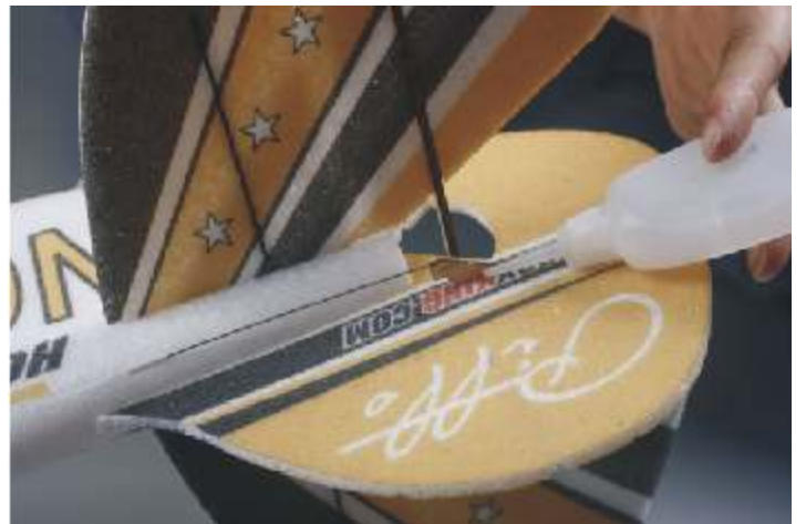
23. Connect another Z wire 0.8*360mm to the horn for rudder pushrod, put the wire through the tube in the fuselage. Press the horn into the slot in the rudder, using CA glue.
