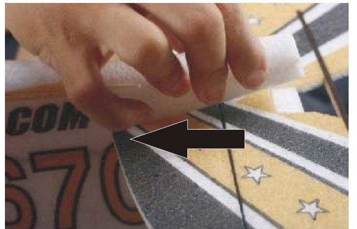
16. Insert the horizontal stabilizer into the fuselage as shown.
