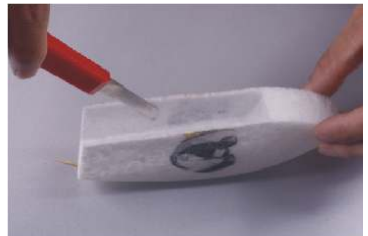
52. Hollow out the canopy with sharp knife and make enough space for servo arm working
