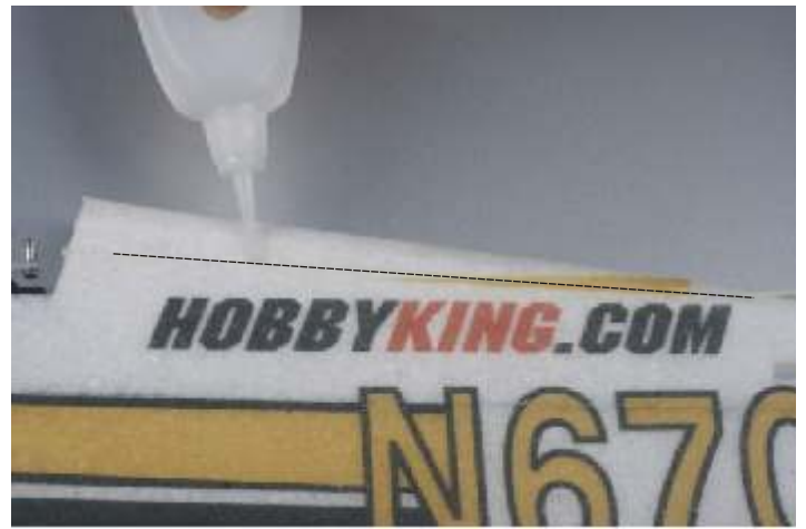
14. Press the tube into the slot in fuselage as shown .glue it using CA glue .
