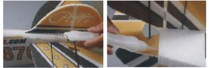
21. Glue vertical fin on the fuselage using CA glue. check the perpendicularity and alignment as shown.
