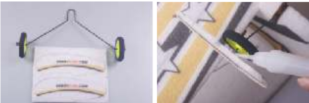
56. Insert the landing gear into the fuselage. Fix the wheel covers with some CA glue.
