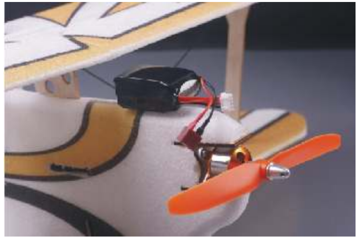
59. Moving the accu pack make the model balance . cut opening In the fuselage for accu pack –the hole must be about 1mm smaller of each side ,the fuselage foam will hold the accu pack in the right position.
