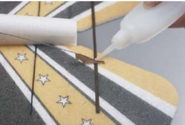
19. Connect the Z wire 0.8*360mm to the horn (with slot) for elevator pushrod, and ensure the wire through the tube in the fuselage. Press the horn into the slot for the elevator, using CA glue.
