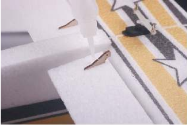
39. Glue the control horns into the ailerons with CA glue as shown .
