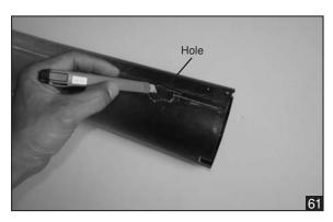
2. Slide the air outlet to the fuselage.
