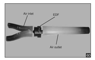
1. Trim 1 hole from the air outlet for the wires of EDF.
