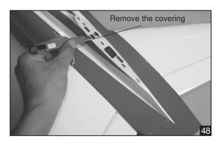
9. Install the vertical stabilizer and glue it using epoxy glue.
