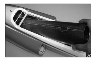
3. Slide the air inlet to the fuselage.
