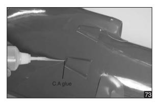
13. Glue the wooden plate onto the vertical stabilizer.
