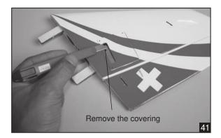
3. Install the rudder servo.
