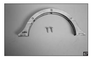
7. Secure the belt to the fuselage.
