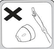
**NEVER** use damaged or deformed propellers or spinners.
