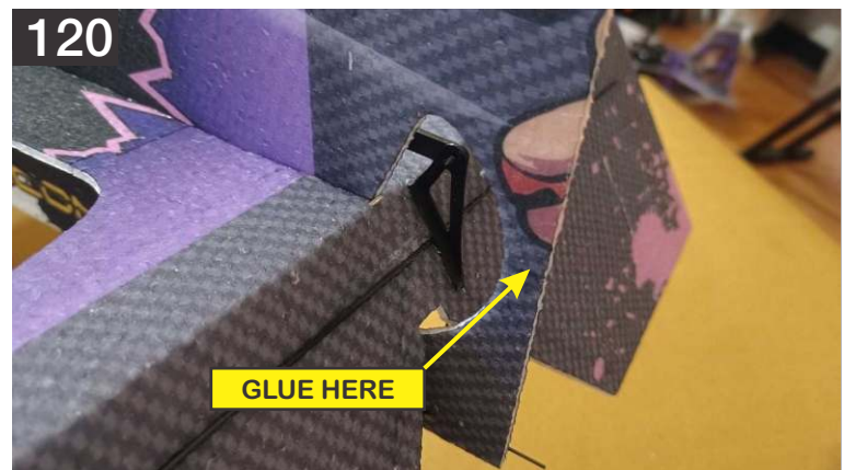
120. Note that there is a small area behind the elevator that should mate up as well.
