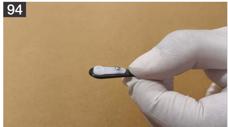
94. Install the extenders over the stock plastic servo arms using the small screw. Wrap with thread for more strength if desired
