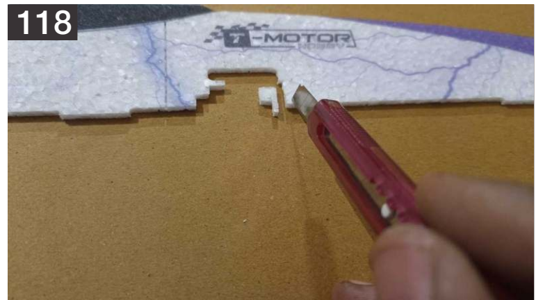
118. Dry fit the top part of the fuselage, trim any slots if needed.
