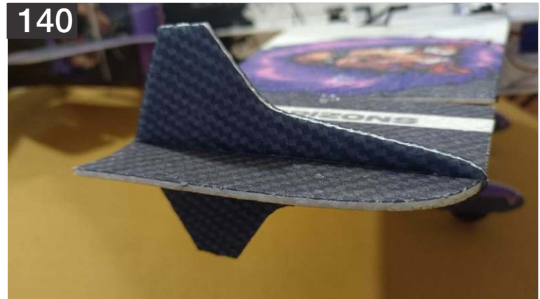
140. Test fit it into the slots on the ailerons. Sometimes a little trimming is needed. Once happy with the fit use either thin CA or HV CA to attach the piece.
