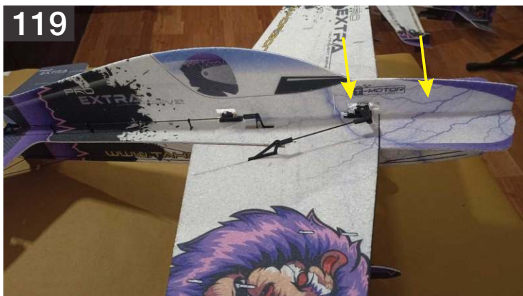
119. Once the aileron and elevator linkages are set up, use the same process as gluing the bottom of the fuse to glue the top of the fuselage into place. Engage all the tab and slots. Press firmly along the length of the fuselage to make sure all areas are fully seated. Check that the top piece is square and straight. Tweak if necessary to make it true.
