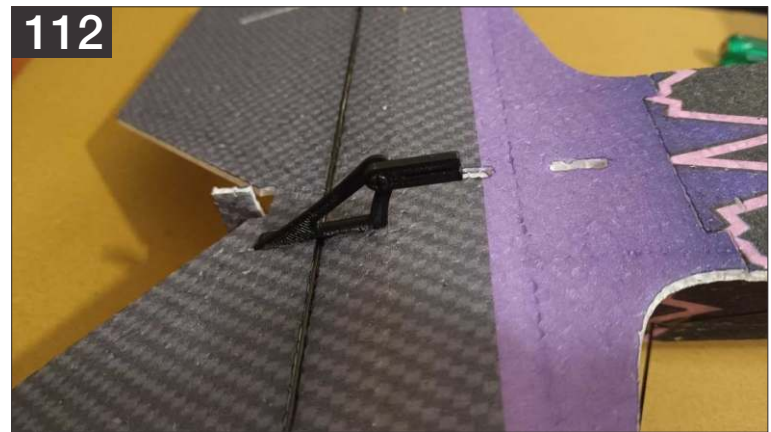
112. Screw the 1.2mm dia control links over the both elevator control horn and servo arm as shown above.
