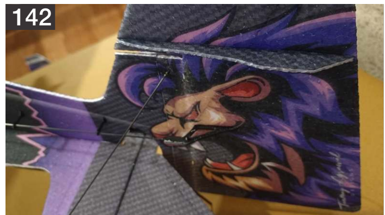
142. Test fit it into the slots on the rudder. Sometimes a little trimming is needed. Once happy with the fit use either thin CA or HV CA to attach the piece.
