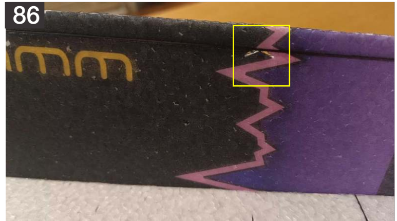
86. Up Next is the fuselage trussing. Locate the pre cut small slots all over the tail, horizontal and vertical profile sections.
