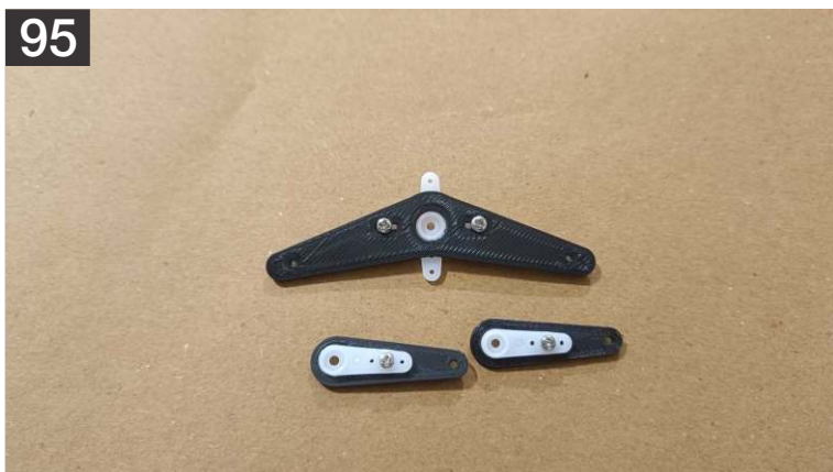
95. Here are all servo arm extenders are installed over the stock servo arms.
