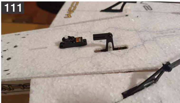
111. Elevator linkage, Make sure you have the servo centered before moving further with the setup, check the orientation shown in the above image.
