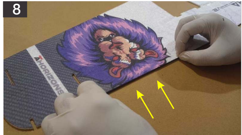
8. Apply a thin layer of HV Cyno on CF Spar, and glue it on the leading edge of wing, like shown above.
