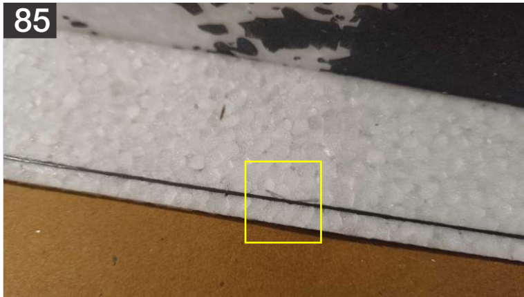
85. Up Next is the fuselage trussing. Locate the pre cut small slots all over the tail, horizontal and vertical profile sections.
