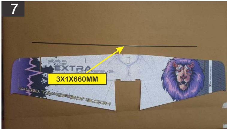
7. Locate the 3mm X 660mm CF Spar shown in the picture above
