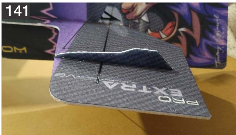
141. Test fit it into the slots on the elevators. Sometimes a little trimming is needed. Once happy with the fit use either thin CA or HV CA to attach the piece.
