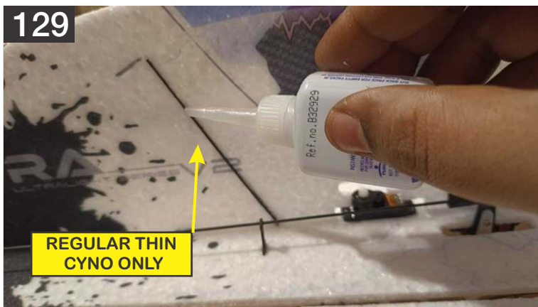
129. Use a thin cyano and activator to glue it.
