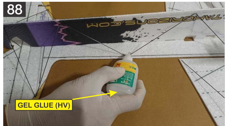
88. Carbon rod needs to sit couple of mm into the pre cut slot into the foam before gluing, Just put a small drop of HV Cyno to glue it.
