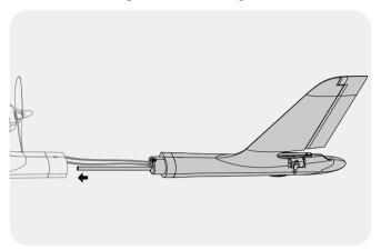
2. Secure the joint of the front and rear fuselage using included screw.
