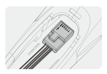
2. Tear off the adhesive sticker on the back of Vector unit and stick the Vector unit to the position as shown in the below figure.
