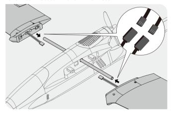
3. Secure the wing set using included screws as shown.
