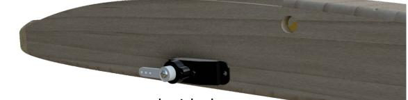
The Pictheron servos are mounted with the Servo output spline toward the nose and the output arm parallel with the servo body as shown above. Use the longest arm possible that is supplied with the servo. Its surprising how much movement you need on the wing particularly for pitch control.
