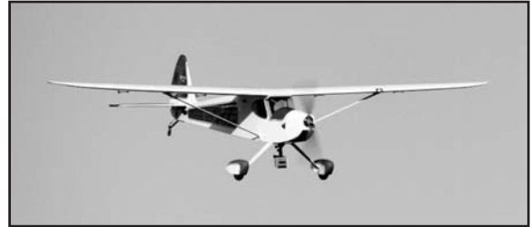
Here is another Rascal 110 with an onboard camera, this time mounted on the bottom between the landing gear legs.
