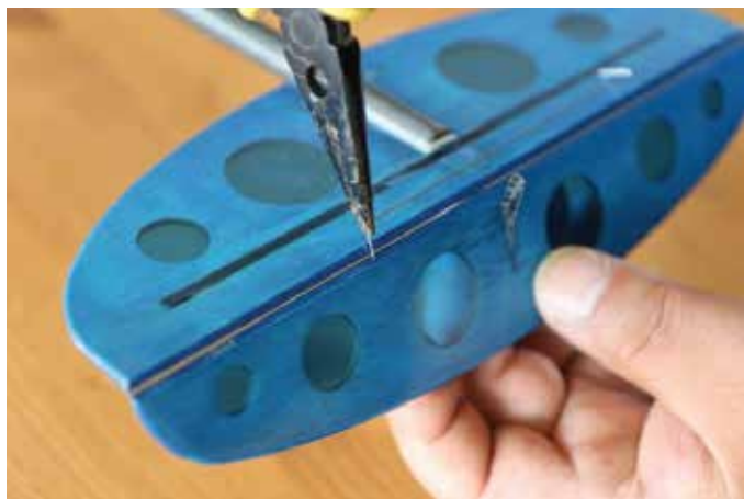
24. Insert and glue one end of the torsion spring into the rudder hinge slots as shown.
