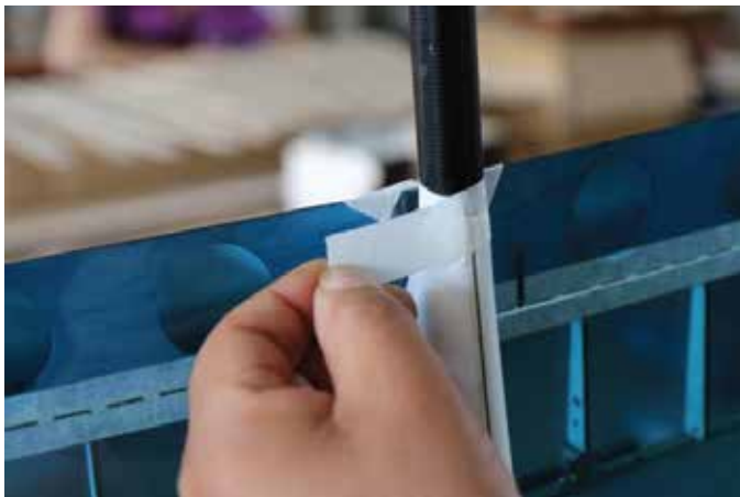
19. Once satisfied with the tail boom alignment, use paper tape to secure the tail boom in place and wait for the glue to dry.
