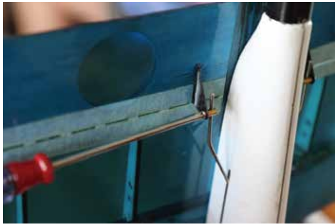
34. Install the aileron pushrod to the pushrod adjuster as shown.
