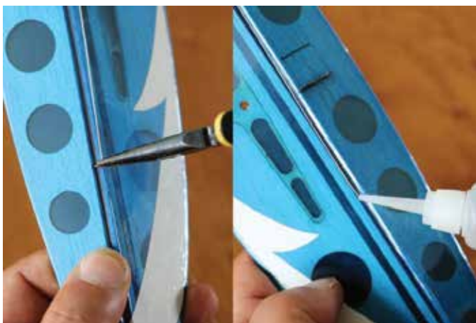
26. Use the same method as shown above to install the torsion spring on the elevator.
