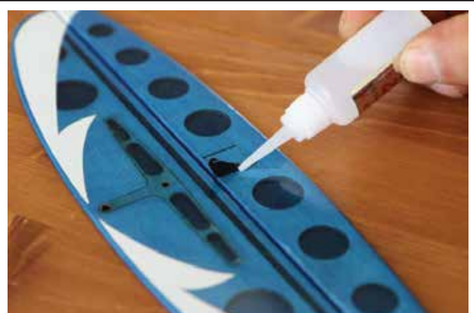
21. Glue the elevator horn as shown.
