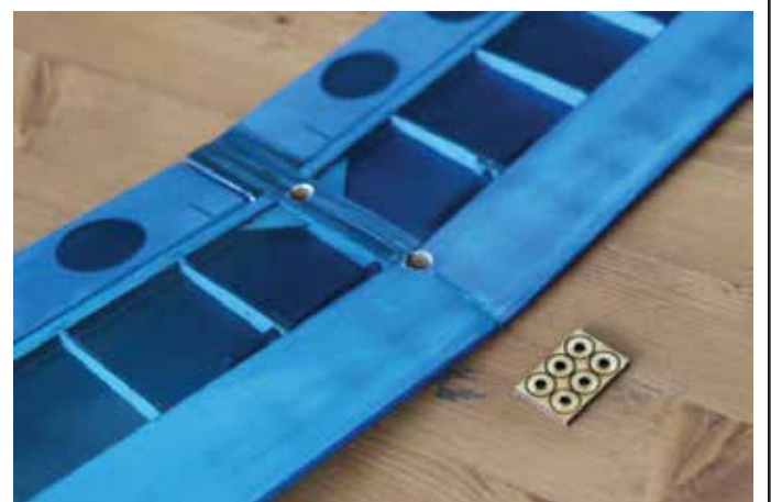
14. Install the shims after the glue has been completely cured.
