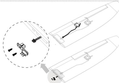
7. In case you ordered the KIT version, or you need to change a servo: Simple remove the screws that hold the servo connectors on the wings, disconnect the old servo and connect the new one, re-routing the cable in the same way it was before, screw the assembly back on and you are ready.
