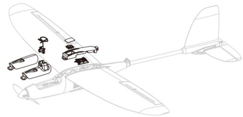
4. Install all your gear: Radio Rx, flight controllers, battery, etc. Check that all your surface are moving correctly before going to fly.
