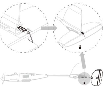
1. Install the horizontal stabilizer and make sure you are matching the hole on the tail section. Use the provided thumbscrew to lock the horizontal stabilizer in place. Connect the clevis to the hole of the control horn.
