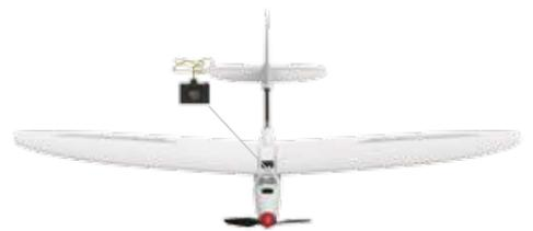
6. The extra FPV hatch can host most AIO cameras on the market and micro HD as well.
