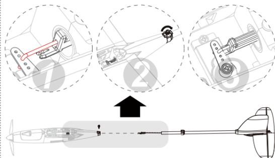
2. Install the tail boom following the graphics. The pushrod goes in the middle hole of the servo arm. Don't forget to lock the clevis against the pushrod when you are set. The tail should align perfectly with the motor. Once all is connected, lock the plastic part to hold the boom in position.
