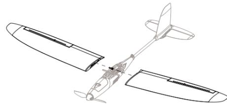
3. Insert the carbon fiber rod in the fuselage, and then connect the main wings, making sure both are touching the fuselage, then lock the main wings with the thumbscrews.
