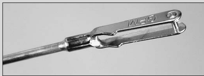
This is what a properly soldered clevis looks like—shiny solder with good flow, no blobs, flux removed.
