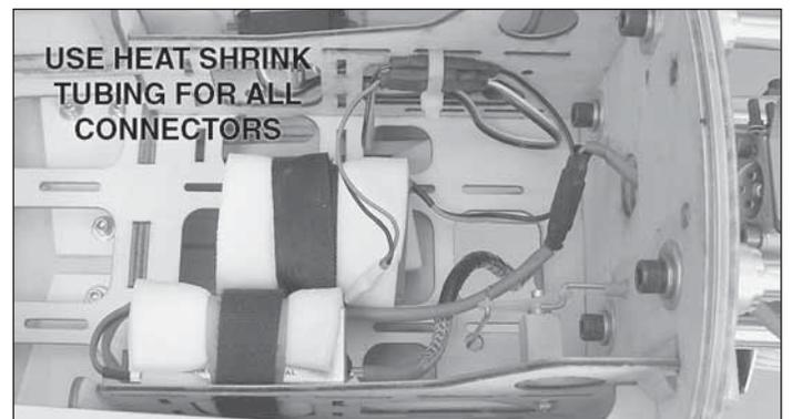
❑ 25. Connect the ignition module to the ignition switch. Connect the crank pickup to the ignition module. Connect the ignition battery to the ignition switch. Use heat shrink tubing to secure the connectors and a tie wrap to secure them to the upright.
