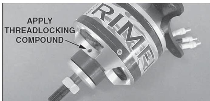
2. Prepare your motor by removing the motor mount screws, the two forward motor case set screws, and the rear locking collar set screw. Apply threadlocking compound to these and reinstall them.
