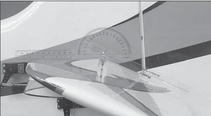
Use a ruler, an inclinometer, or a protractor to accurately measure and set the control throw of each control surface as indicated in the chart that follows. If your radio does not have dual rates, we recommend setting the throws at the **high rate** setting.
