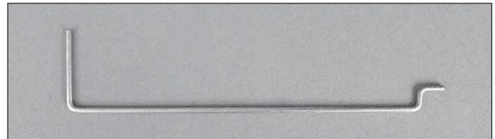
❑ 9. Make a Z-bend at one end of pushrod B and a 90° bend at the other end as shown. The last 3/4" [19mm] of rod should be left for the 90° bend.
