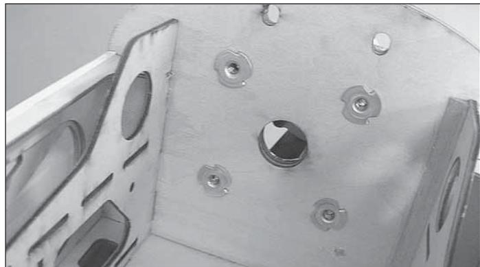
❑ 3. Press four 8-32 blind nuts into the engine mount holes you drilled. Press them in from the back side of the firewall. You may need to use 8-32 bolts and washers to draw the nuts into the holes.
