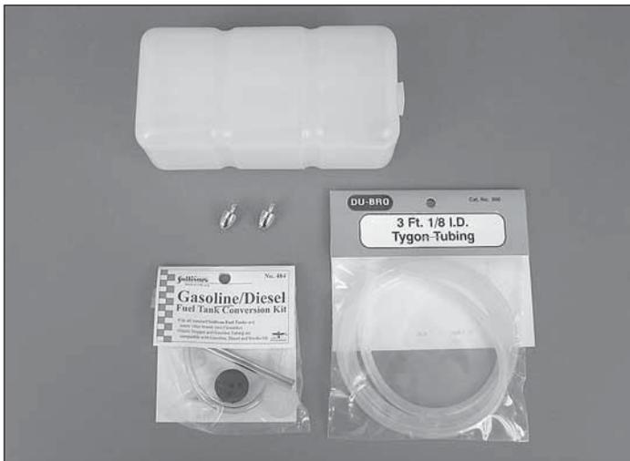
□ 27. The fuel tank hardware that is supplied with this kit is **suitable for glow fuel only and cannot be used with gasoline**. For this reason we recommend the Sullivan gasoline conversion kit (SULQ2684), five fuel line barb (2x DUBQ0670), 36" [914mm] of Dubro 1/8" [3mm] Tygon fuel tubing (DUBQ0493), and 24" [610mm] of Dubro neoprene gas fuel line (in-tank) (DUBQ0455). Please retain the plastic tank and the fuel clunks. These are approved for gas.
