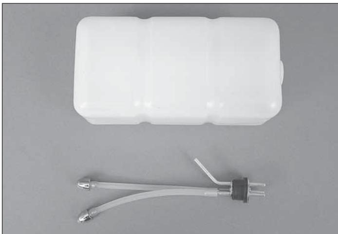
❑ 15. Cut two pieces of fuel line so that each one is 5" [127mm] long. Build up the fuel tank as shown with the vent
