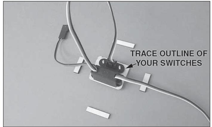
❑ 16. Locate the switch plate that fits your brand of radio switch. Four plates are supplied: two Futaba switch & Ernst charge jacks and two Hobbico heavy-duty & Ernst charge jacks. Fit your switch and charge jack to the plate and use a pen or pencil to draw an outline of the switch and jack onto the back side of the plate. Remove the switch and charge jack.
