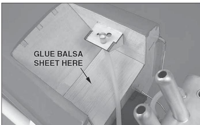
20. Test fit the covered balsa sheet as shown. The sheet is not "square." It matches the angle of the firewall. **Note:** One side has clear covering which must face outward.
