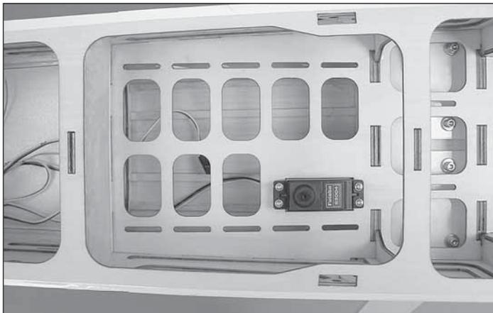
❑ 6. Install the throttle servo in the center equipment tray as shown. Use a 1/16" [1.6mm] drill bit for the servo screw holes.
