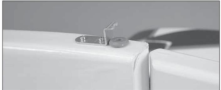
❑ 5. Use the two 8mm sheet metal screws to attach the retainer to the fuselage.
