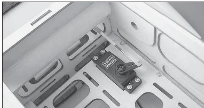
❑ 10. Install a servo arm. Set your throttle servo to the full-throttle position and connect the pushrod.
