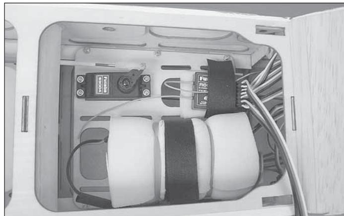
❑ 16. Wrap your receiver and battery pack with 1/4" [6.4mm] thick latex foam. Use the straps you made to mount your battery and receiver to the aft equipment tray.
