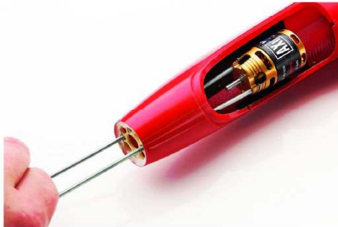
Pro snadné vsunutí motoru do trupu si pomozte dvěma kousky závitové tyče. Help with two pieces of threaded rods for easy insertion of the motor into the fuselage.
