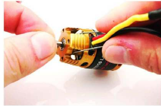
Vsuňte pružinku do motoru. Insert the spring into the motor.
