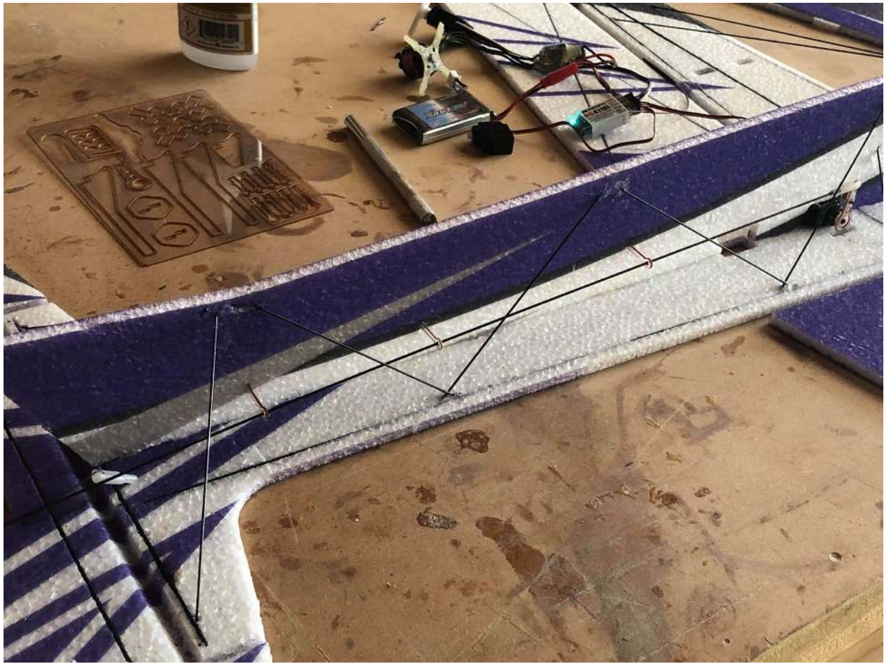
Shown above is the bottom fuse bracing for the rear of the fuselage. Lengths found in diagram.
