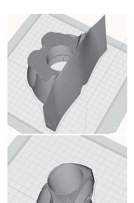
The following parts must be sliced with the PROFILE P5\_GYROID. Please note the additional settings for the individual parts! It is essential to print these parts with LW-PLA!
