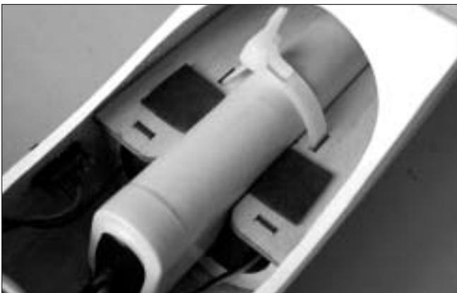
44. Apply furnished foam tap on battery mount, it will help retaining the battery pack in place.
