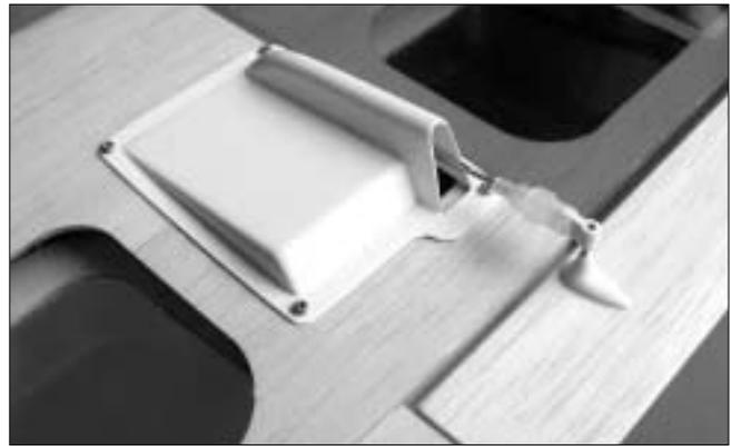
14. Next secure the Hatch Cover in place with furnished 2x5 mm wood screws. Snap on the clevis on control horn. Thread a small piece of silicone tube and slide it on the clevis to prevent it from loose.
