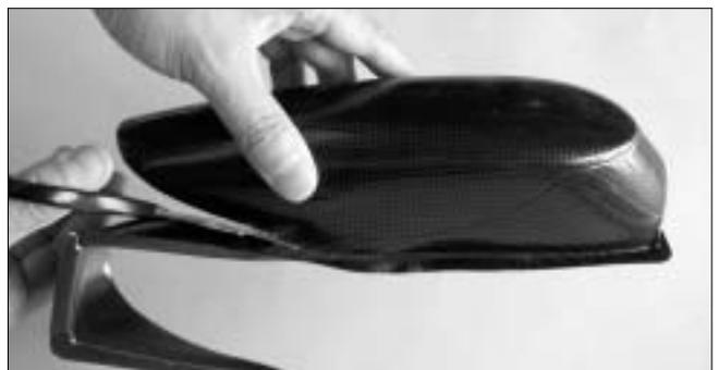
46. Locate the canopy. Cut 1/16" (1.5mm) outside the molded line with curved scissors. Trial fit and trim it until it fits on the fuselage.
