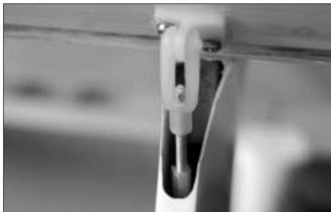
34. Snap the clevis onto the control horn as shown. It may need to file the T-Tail portion to make sure the movement is free.
