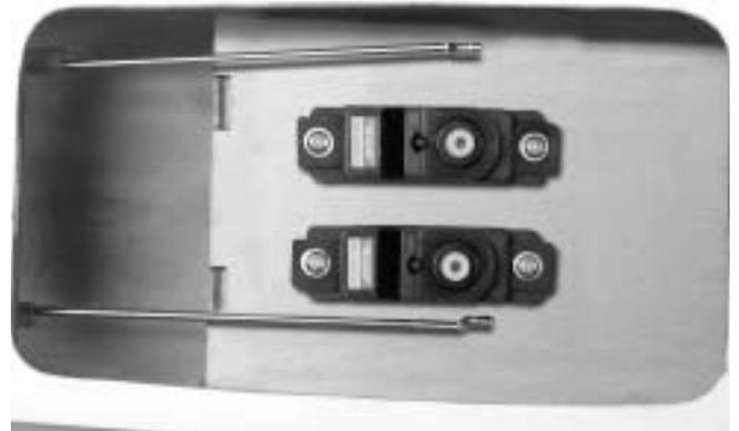
40. What we used here are mini servos. You may use standard servo but need to enlarge the servo tray. The upper one is elevator servo and lower one is rudder servo.
