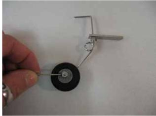
$\square$  step 4 Locate the tail wheel on rudder and glue it with some drops of medium CA.
