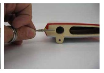
$\square\square$  step 3 Place the three hinges in their holes, and verify the correct position and alignment of the elevator with the stabilizer panel.
