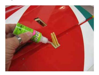
$\square\square$  step 4 Drill the location for the four self-tapping screw using a 1.5mm drill bit and install the servo into the wing panel as per the picture.
