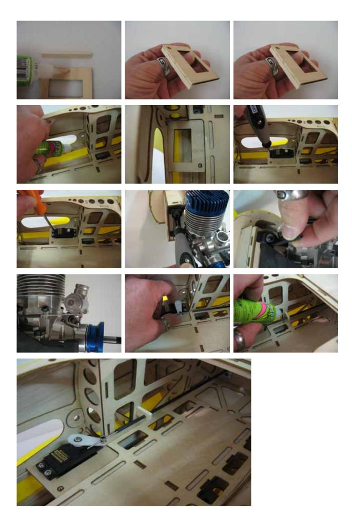
$\hfill \square$  step 8 Assemble and locate the tank as follow.
