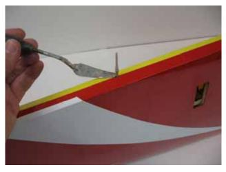
□□ **step 3** Carefully glue, with 5 minutes epoxy, the hinges into the aileron.
