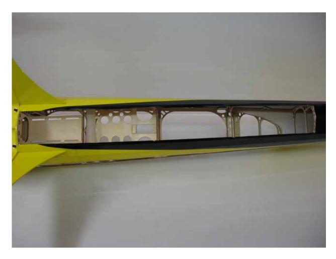
$\Box$  step 2 Install and glue all the tunnel pipe's parts with medium CA, as follow.
