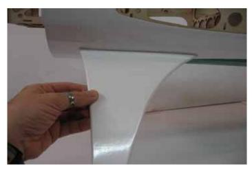
□□ **step 7**Once satisfied with the fit, glue the fillet on the landing gear using medium CA. Use the glue carefully avoid over runs on other areas.
