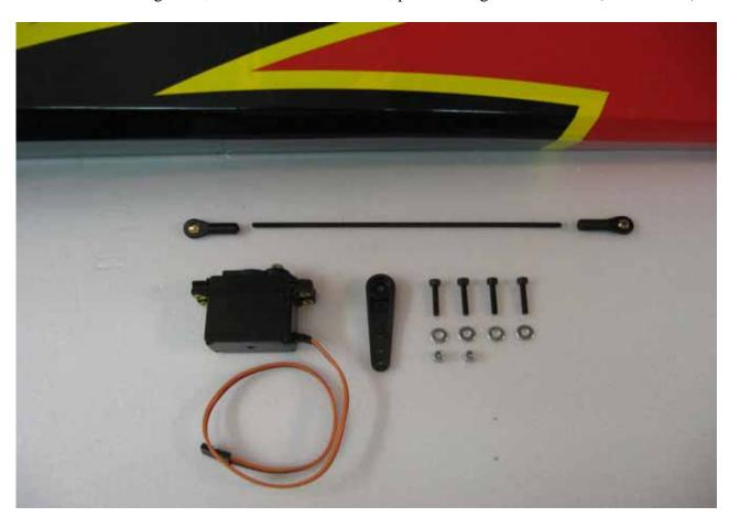
$\square\square$  step 2 Drill the location for the four self-tapping screw using a 1.5mm drill bit and install the servo into the wing panel as per the picture.
