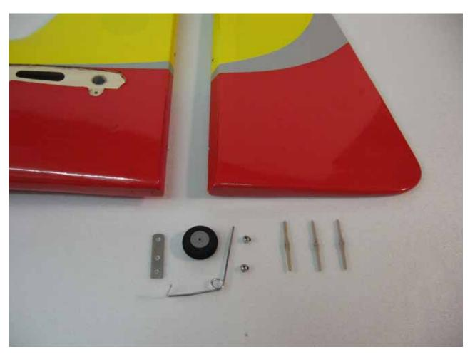
$\Box$  step 2 Using a 2mm drill bit, carefully drill the hole into rudder, 25mm from the base level, for the tail wheel. With the hobby knife cut a groove 25mm length into the rudder as follow.
