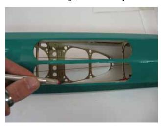
$\square$  step 6 Apply a piece of masking tape on the line were you have to make the top hole for the cowl fixing screw, and mark the position as per the picture.
