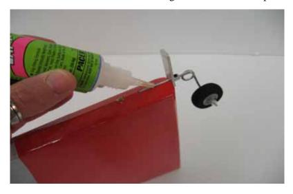
$\square$  step 5 Prepare the hinges for the application, using one small drop of sinthetic oil in their center of movement.
