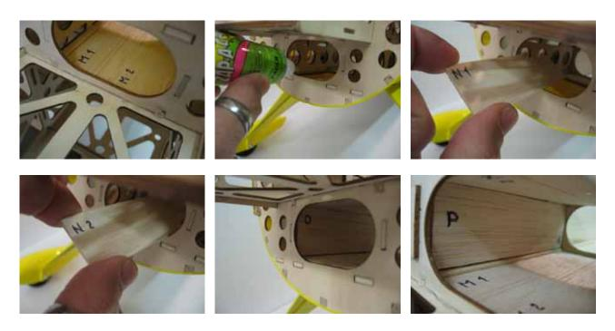
$\hfill\Box$  step 5 Locate and glue the motor mount reinforcement parts with medium CA, as follow.
