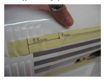
$\square$  step 12 Drill the location for the four self-tapping screws using a 1.5mm drill bit. Attach the cowl using the four self-tapping screws, included in hardware pack, and a Phillips screwdriver.
