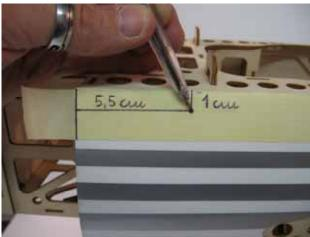
$\Box$  step 7 Apply a piece of masking tape on the line were you have to make the bottom hole for the cowl fixing screw, and mark the position as per the picture.
