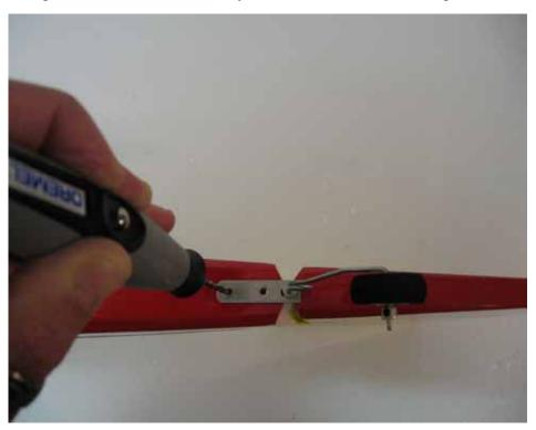
$\hfill \Box$  step 10 Use the two self-tapping screws to fix the tail wheel as follow.
