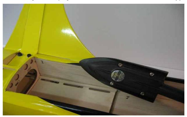
□ **step 4**Install and glue this tunnel pipe's parts with medium CA too, as follow.
