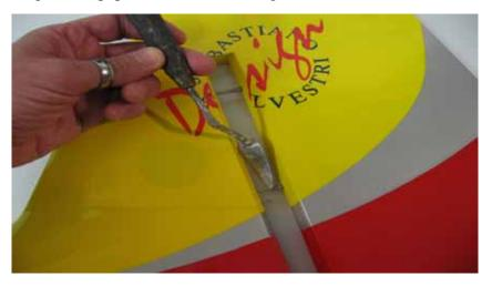
$\square$  step 8 Work the rudder right and left some times to work the hinges and check for proper movement.
