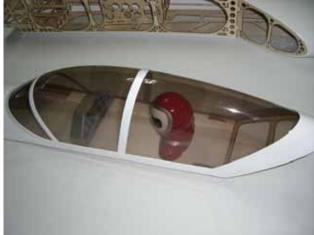
$\Box$  step 4 Locate the canopy on fuselage and place the 3mm screws with washers to fix it, as per picture.
