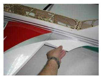
□□ **step 3** Once satisfied with the fit, glue the wing fillet to the wing panel using medium CA. Use the glue carefully avoid over runs onto the area to be covered with the material.
