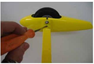
$\Box\Box$  step 6 Test fit the landing gear fillet and his alignment.
