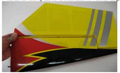
□□ **step 8**With the hobby knife remove the cover in the control horn location.
