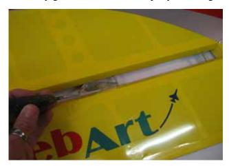
$\Box\Box$  step 4 Work the aileron up and down some times to work the hinges and check for proper movement.
