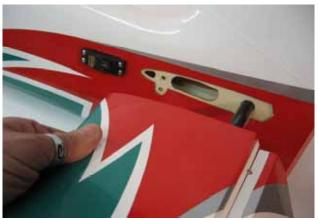
$\Box\Box$  **step 4** Fix the stabilizer on the fuselage with the provided 3mm screws and washers.
