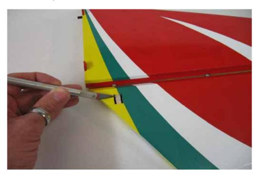
$\square\square$  step 9 Place the fibreglass control horn into elevator, check for correct alignment and glue it with some drops of medium CA.
