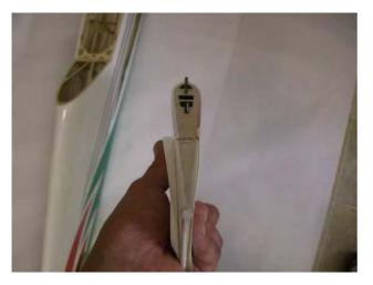
Use the covering iron carefully, at a medium temperature, to glue the cover material down around the area of the fillet. Use caution while working around areas where the cover material overlaps to prevent separating the covers.
