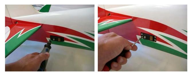
Glue the fibreglass horn with medium CA into the rudder. Than install the hardware and make the final adjustment as per picture.
