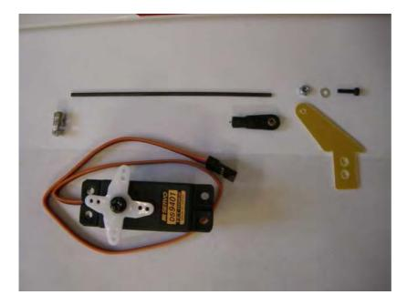
Install the servo hardware (gommets and eyelets) and put the servo into the wing panel, as per pictures.
