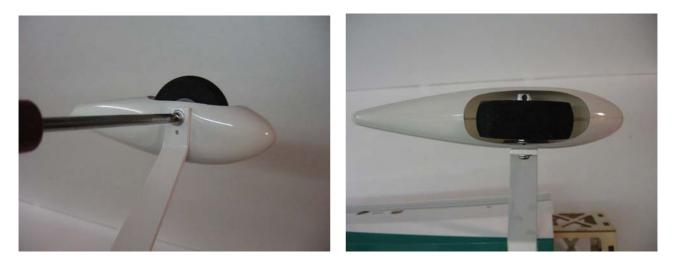
Drill the location for the wheel pant fixing screw using a 1,5mm drill bit and than fix the wheel pant with the screw included in the hardware pack.
