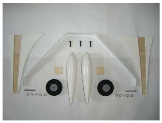
Locate the landing gear on the fuselage and fix it with the screws included in the hardware pack.
