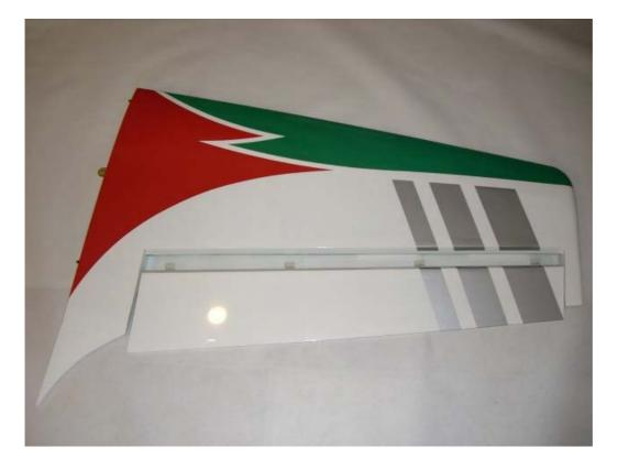
Carefully glue, with some drops of thin CA, each of the four hinges in the aileron.
