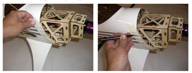
Slide the cowling onto the fuselage and install the spinner back plate. Then apply another piece of masking tape on the same line of the one applied before. Drill the location for the four self-tapping screws using a 1.5mm drill bit.
