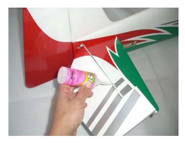
Locate the carbon tube in his position and carefully check the alignment of the stabilizer with the fuselage, as per pictures.
