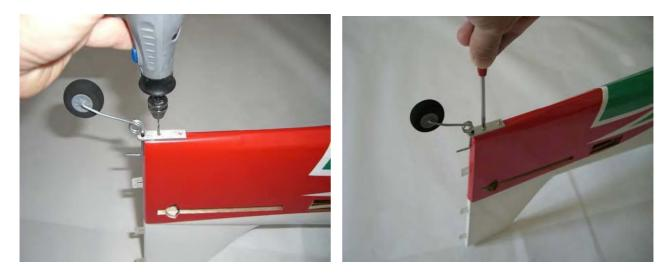
Carefully put some drops of medium CA into the 2 mm hole, carefully locate the rudder and glue the hinges with some drops of thin CA.
