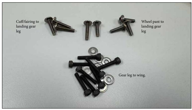
Attach the gear legs to the wing mount so that the gear sweeps FORWARD. Use blue threadlocker. Install the cuff/ fairings as shown with threadlocker. Install the axles with washers and locking nuts, point the flat spot on the end of the axle DOWN toward the runway. Install the wheel and the wheel collar, tightening the set screw against the flat with threadlocker. Install the wheel pants as shown, using threadlocker.
