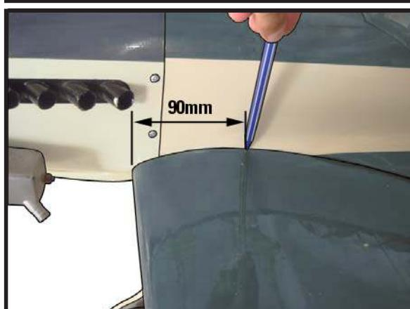
1) It is critical that your airplane be balanced correctly. Improper balance will cause your plane to lose control and crash. The center of gravity is located 90mm back from the leading edge of the wing, measured at the wing root.
