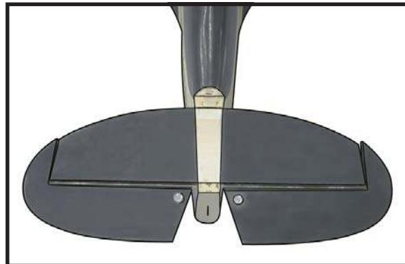
9) When you are sure that everything is aligned correctly, mix up a generous amount of 30 Minute Epoxy. Apply a thin layer to the bottom of the stabiliser mounting area and to the stabiliser mounting platform sides in the fuselage. Put the stabiliser in place and realign. Double check all of your measurements once more before the epoxy cures. Hold the stabiliser in place with T-pins or masking tape and remove any excess epoxy using a paper towel and rubbing alcohol.
