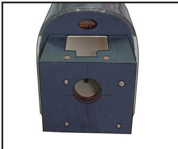
3) Attach the motor to the front of the electric motor box using four 3mm blind nut, four M3x15mm hex head bolts to secure the motor . Please see picture shown.
