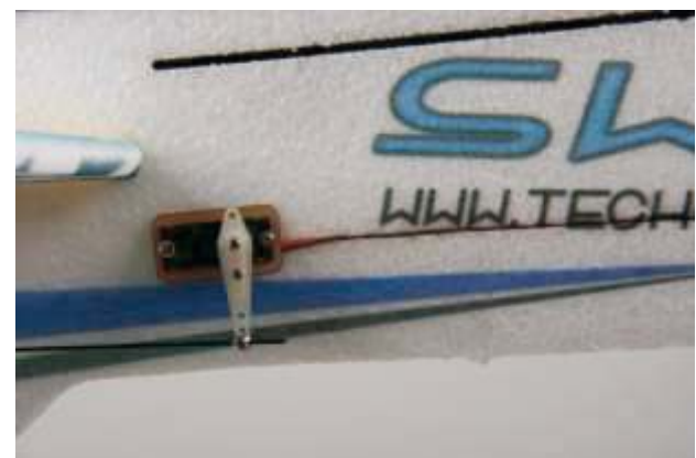
33. Embed the rudder and elevator servo leads into the pre-cut slots on two sides of fuselage. Pls use the servo extension wire if the servo wire is not long enough.
