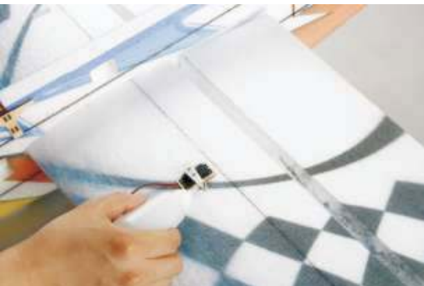
10. Put the servo into the pre-cut servo hole, then use glue to fix the servo mount onto the wing. Make sure the servo arm point to the wingtip.
