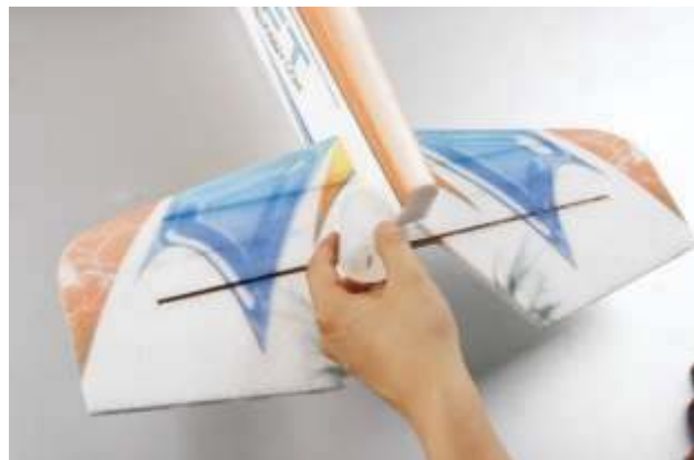
22. Drop some glue on the joints of elevator and fuselage to fix.
