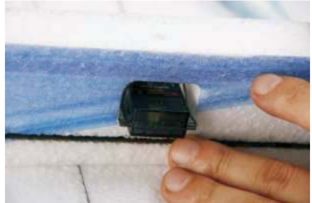
40. After test, put the receiver into the receiver slot. (see picture)
