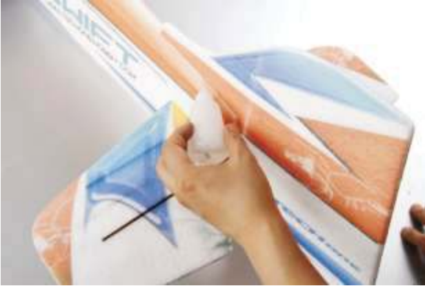
23. Use CA to fix the rudder.
