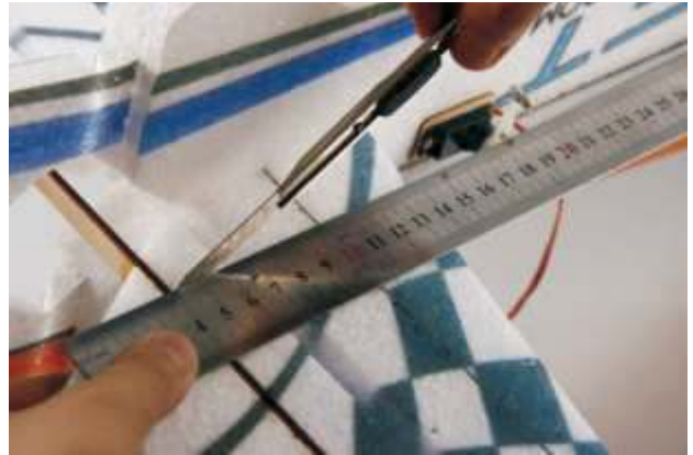
26. Use a hobby knife to cut a small slot on the elevator so that can install the control horn easily.
