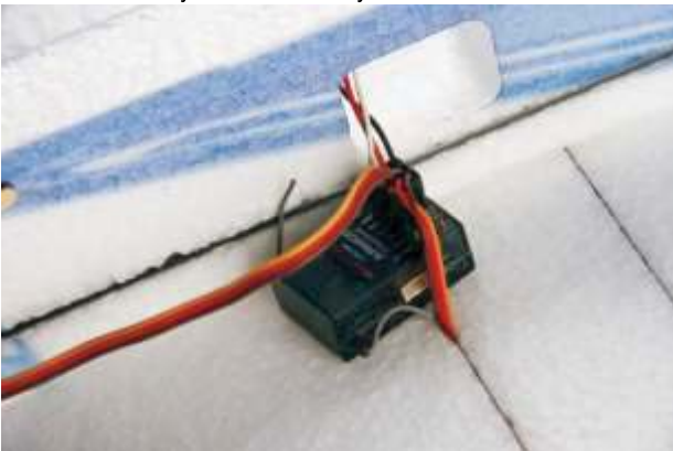
39. Link the servo leads and ESC to receiver, then test.
