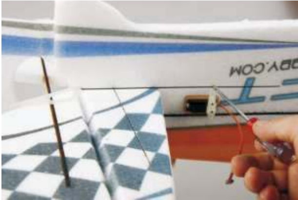
30. Use screwdriver to tighten the pushrod connector with the screws.
