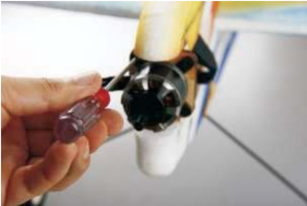
36. Use included screws to fix the motor onto the motor mount.
