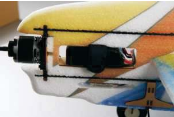
38. Insert battery into the battery hole.
