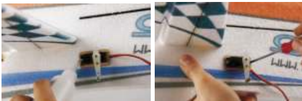
31. Use the pinchers to cut off the superfluous steel wire.
