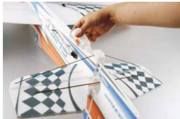
34. Connect the horizontal stabilizer to the bottom of the fuselage by using 2pcs 1.3*230mm stab brace carbon rods, and then reinforce the rods by using CA, pls make sure the Horizontal Stab is vertical the fuselage when you connect.
