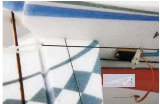
28. Through the other side of the Z bend to the hole of pushrod connector , and then insert the rudder and elevator horn into the pre-cut slot.
