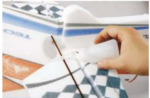
29. Glue the control horn
