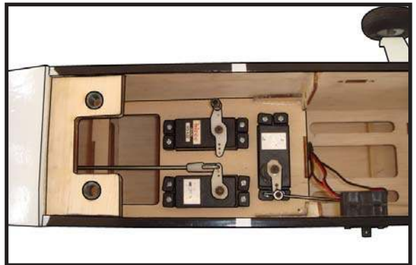
RUDDER PUSHROD HORN INSTALLATION.
