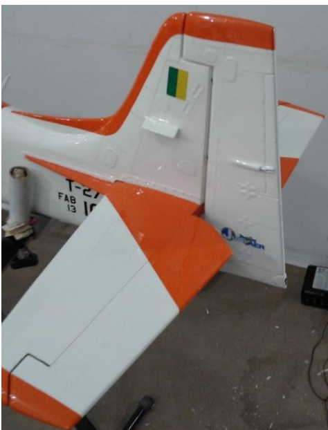
Above: stabilizer and rudder in final position (left) and rudder and elevator control horns (right).
