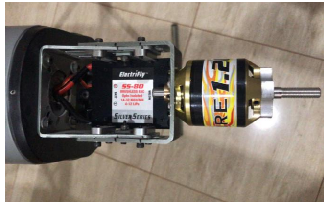
Above: Rimfire 1.20 brushless electric motor on Great Planes adjustable motor mount.
