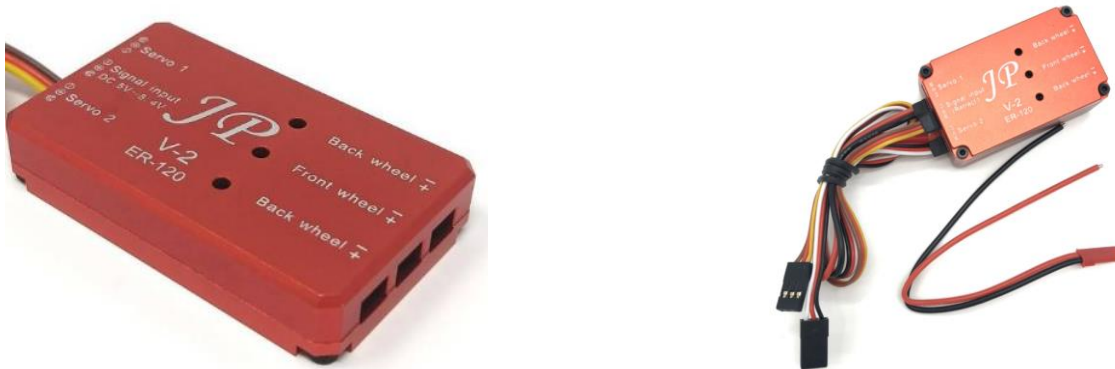
Above: JP ER-120 V2 controller showing retracts connections (left). Power wire (red and black) retracts radio signal wire (yellow, red and brown) (right).
