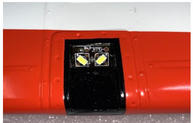
Above: Correct locations for fixing wingtip light boards (left) and landing lights (right).
