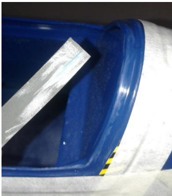
Above: Sand the contact area of the frame to increase glue adhesion (left) and apply white glue to the entire contact area (right).
