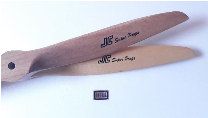
Above: 2 blade wooden propellers for gas burning 20cc engines 14x10 or 15x8.
