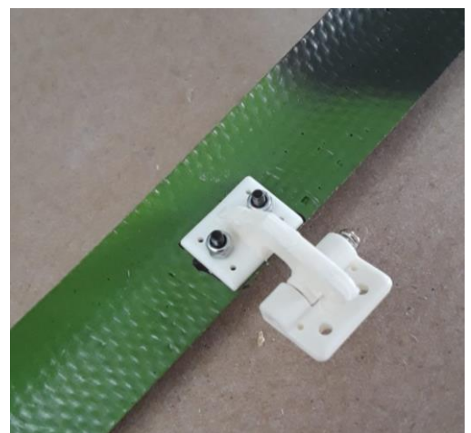
Above: Fixing of the internal hinges for the side opening of the canopy.
