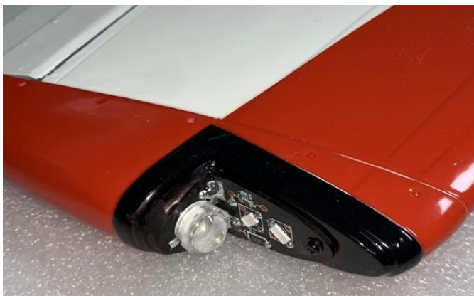
Above: Correct locations for fixing wingtip light boards (left) and landing lights (right).
