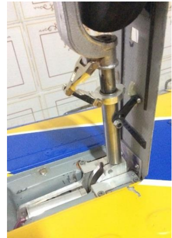
Above: Detail of the attachment of the hinged brackets to the external landing gear door and the closed external landing gear door.
