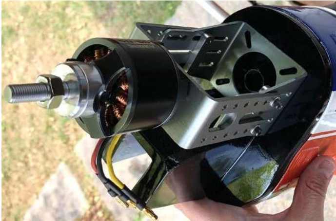
Above: electric motor on Great Planes adjustable motor mount (left) and with custom made stand-offs (right).
