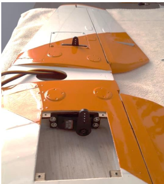
Above: Servo position on the stabilizer rib (left) and elevator servo extensions passing through the lower center of the stabilizer (right).
