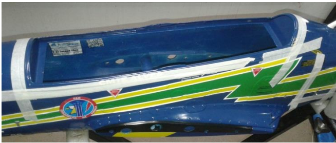
Above: position of the canopy frame on the fuselage and fixing in place with adhesive tape all around.
