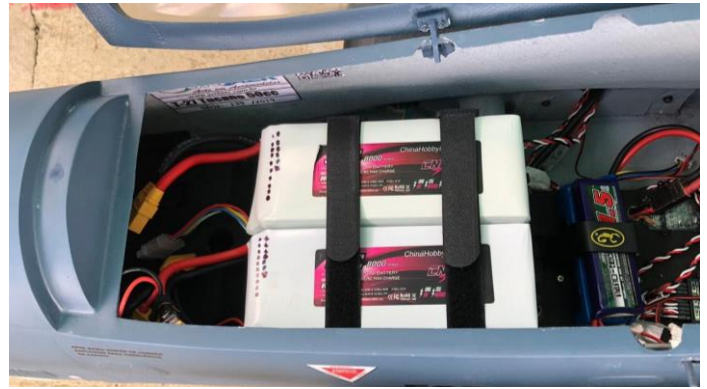
Above: equipment installation examples in the fuselage interior on electric version and Li-Po batteries.
