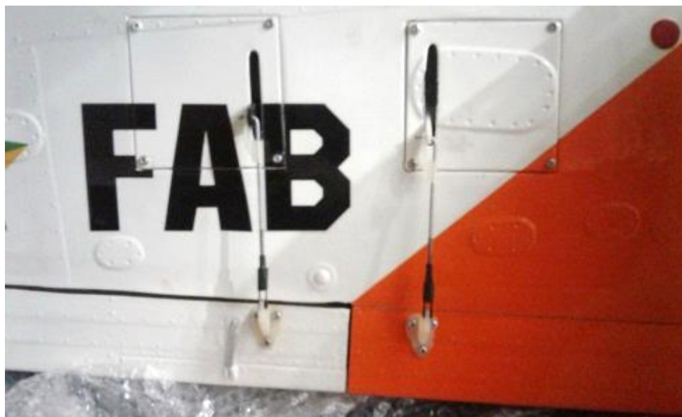
Above: Location of servo access covers, servo arms, horns, and aileron and flap linkage.
