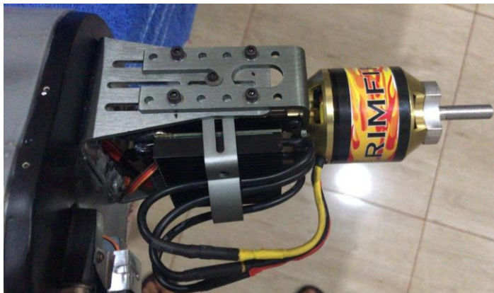
Above: Rimfire 1.20 brushless electric motor on Great Planes adjustable motor mount.
