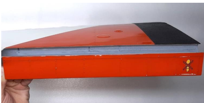
Above: gray areas (trailing edges) on ailerons (right) and flaps (left) shall not be drilled or cut.
