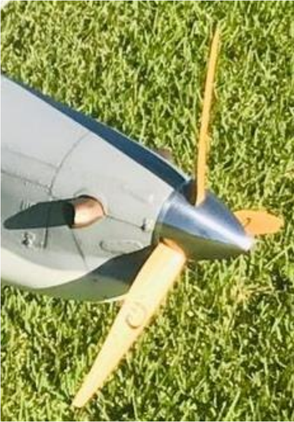
Above: spinner/cowling parallel alignment.
