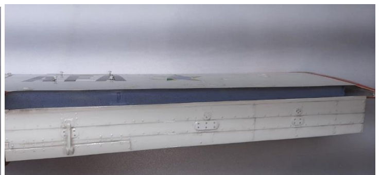
Above: gray areas (trailing edges) on ailerons (right) and flaps (left) shall not be drilled or cut.
