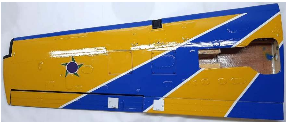
Above: right wing half with servo compartment covers and horns reinforcements places (30mm x 30mm) on aileron and flap marked in white.
