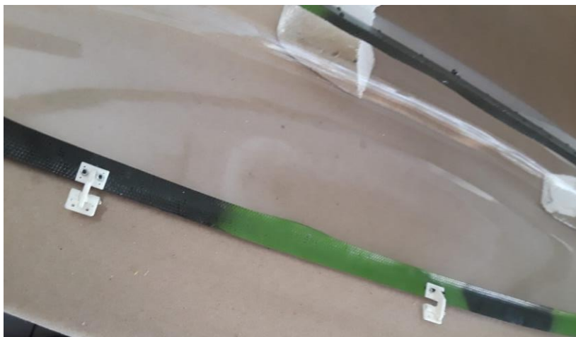
Above: Fixing of the internal hinges for the side opening of the canopy.
