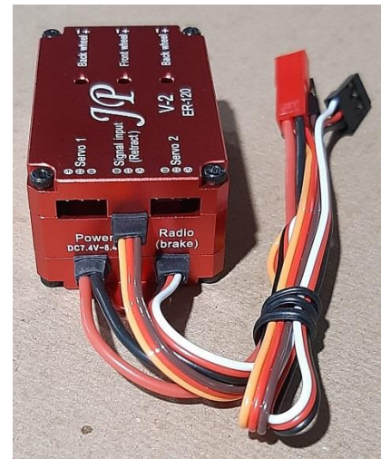
Above: JP ER-120 V2 controller with brakes showing retracts connections on upper side and brakes outputs on lower side (left photo). Power wire (red and black) retracts radio signal wire (yellow, red and brown), brakes radio signal wire (red, black and white) and gear doors servos connections (right photo).
