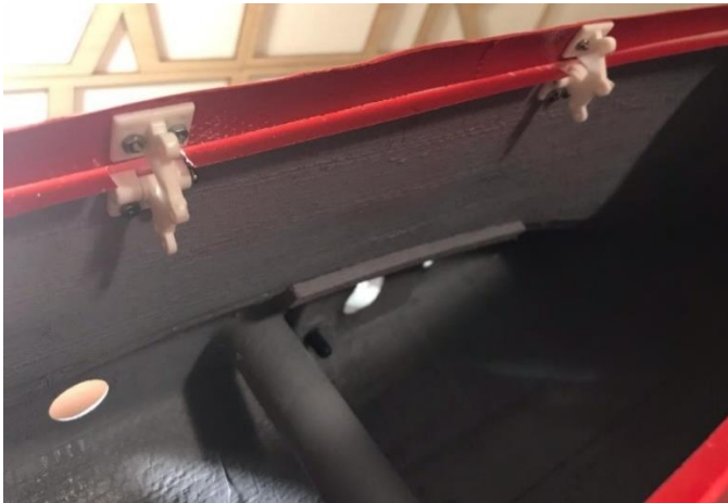
Above: canopy/frame assembly with internal hinges.
