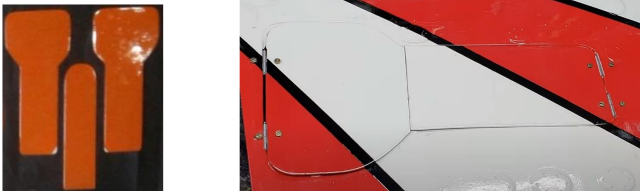
Above: Landing gear door set (left) and main landing gear doors closed with installed hinges (right).
