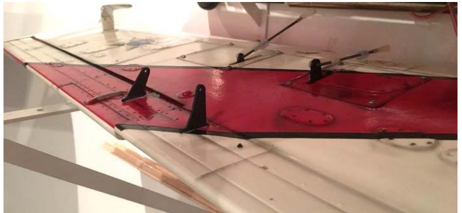
Above: aileron and flap servos installed on the ribs for attachment (left) and position of the horns, servo arms and aileron and flap controls (right).
