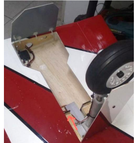
Above: Hinges on door and micro servo installed with linkage.
