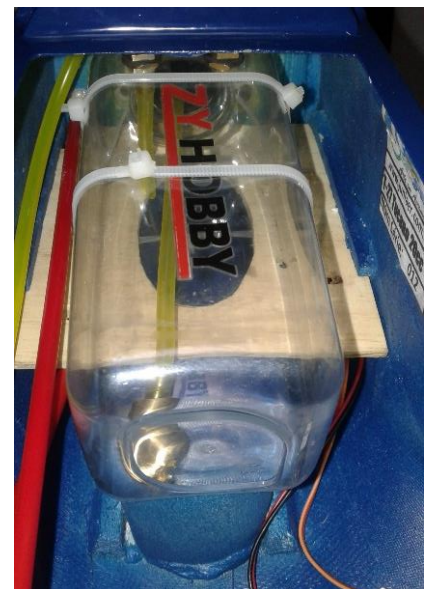
Above: fuel tank with tygon tubes fixed to the fuel tank tray with nylon ties (left) and positioned on rails inside the front of the fuselage (right).
