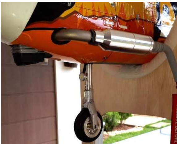
Above: inferior cowling installation with 120 4 cycle glow engine (left and center) and with DLE-20RA muffler exhaust exits and ventilation (right).
