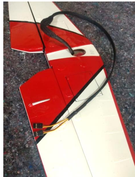
Above: Servo position on the stabilizer rib (left) and elevator servo extensions passing through the lower center of the stabilizer (right).
