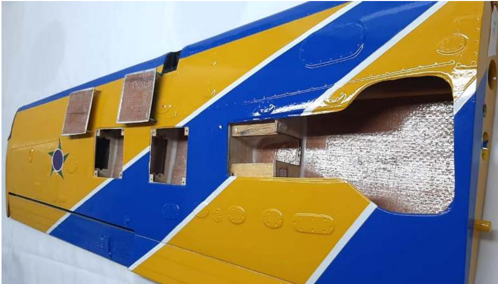
Above: right wing half with open aileron and flap servo compartments showing servo fixation points at the ribs.
