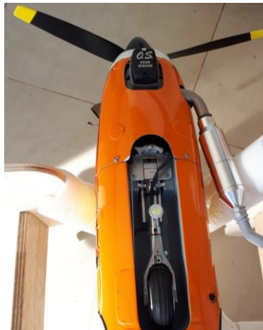
Above: inferior cowling installation with 120 4 cycle glow engine (left and center) and with DLE-20RA muffler exhaust exits and ventilation (right).
