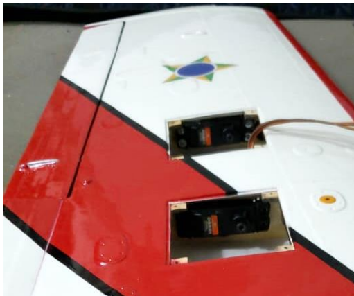
Above: aileron and flap servos installed on the ribs for attachment (left) and position of the horns, servo arms and aileron and flap controls (right).
