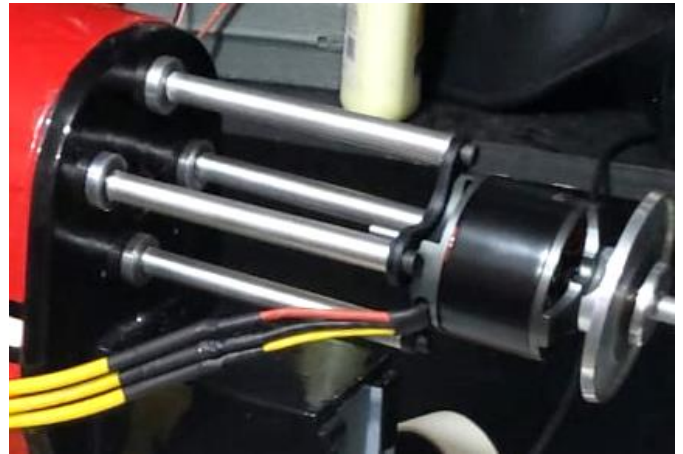
Above: electric motor on Great Planes adjustable motor mount (left) and with custom made stand-offs (right).
