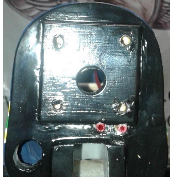
Above: 10-32 blind nuts started to the firewall from the inner side (left) and firewall with the 10mm plywood square part, holes for the engine mount screws, hole for passing the engine spark plug and holes for passage of the engine throttle and choke controls (right).
