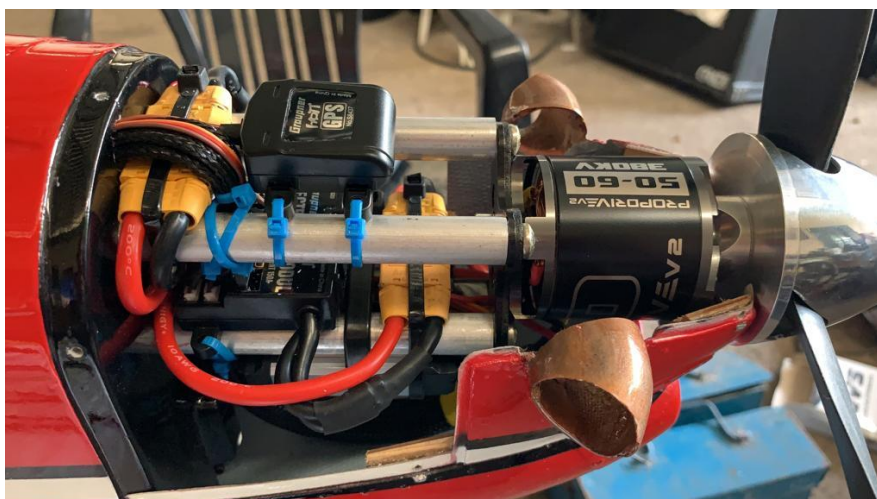
Above: brushless electric motor in custom made stand-offs (right).
