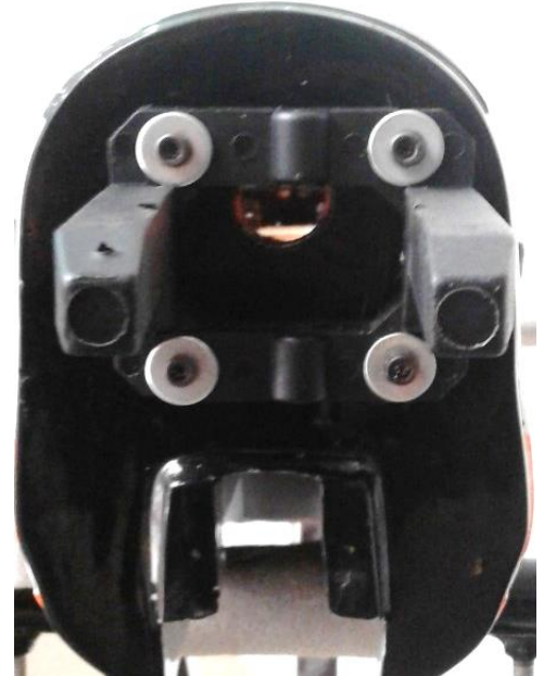
Above: 10-32 blind nuts started to the firewall from the inner side (left) and firewall with screws and washers securing the engine mount (right).
