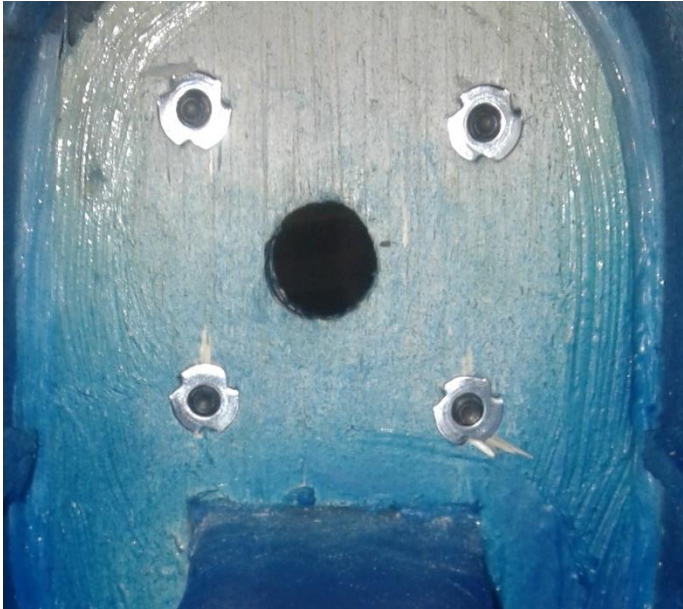
Above: 10-32 blind nuts started to the firewall from the inner side (left) and firewall with the 10mm plywood square part, holes for the engine mount screws, hole for passing the engine spark plug and holes for passage of the engine throttle and choke controls (right).
