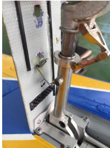
Above: Detail of the attachment of the hinged brackets to the external landing gear door and the closed external landing gear door.
