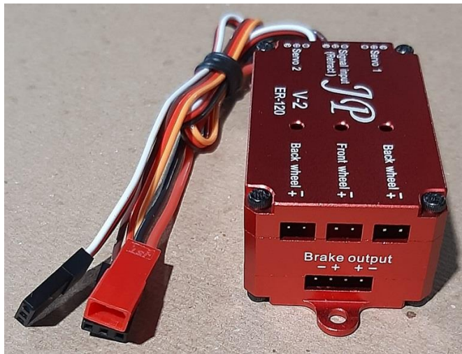
Above: JP ER-120 V2 controller with brakes showing retracts connections on upper side and brakes outputs on lower side (left photo). Power wire (red and black) retracts radio signal wire (yellow, red and brown), brakes radio signal wire (red, black and white) and gear doors servos connections (right photo).
