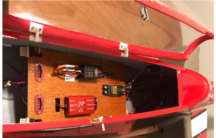
Above: canopy/frame assembly with internal hinges.
