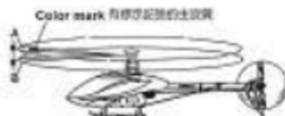
Incorrect tracking may cause vibrations. Please repeat adjusting the tracking to make sure the rotor is correctly aligned. After tracking adjustment, please check the pitch angle is approx. +5~8° when hovering.
