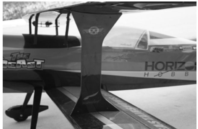
Left interplane strut assembled
