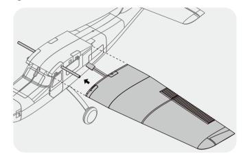
3.Use the included screws to secure the wing halves to the fuselage.
