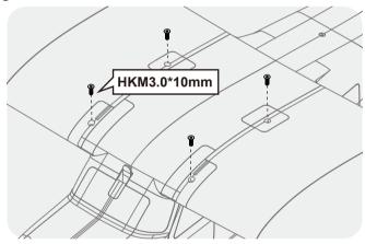
4. Align the holes of support bars with the holes on the fuselage and the main wing. 5. Fix the supporting bars onto fuselage and main wing using included screws.
