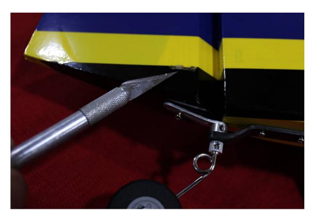
20. Prepare the horn with sandpaper as you did for the wing, and install the rudder horn with 30-minute epoxy as shown.
