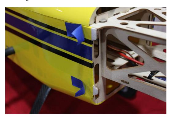
39. Roll the tape back and slide the cowl into position. Install the spinner onto the motor shaft for reference and once satisfied with the cowl position roll the tape back
