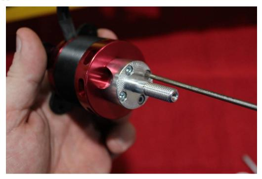
36. Mount the Torque motor using the supplied 4mm black socket head cap bolts and washers. The bolts are to be inserted into the blind nuts which are pre-installed in the motor mount plate. Be sure to put a drop of blue Loctite onto each bolt to prevent them from backing out. Also take time to add CA to all motor box joints!
