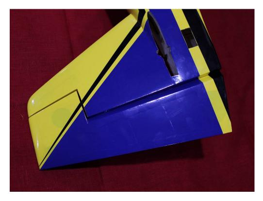
17. Use several drops of thin CA on each rudder hinge.
