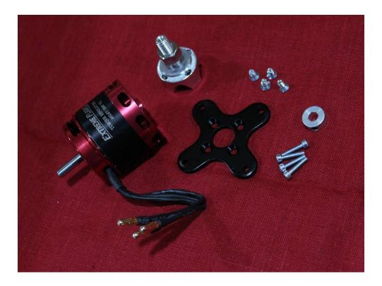
First, slide the provided collar over the motor shaft and secure in place with the set screw. Place a drop of blue Loctite on the threads of the set screw so that it will not back out.
