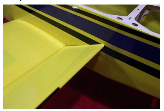
7. Glue the hinges using several drops of thin CA on each hinge. Make sure your thin CA is reasonably fresh.
