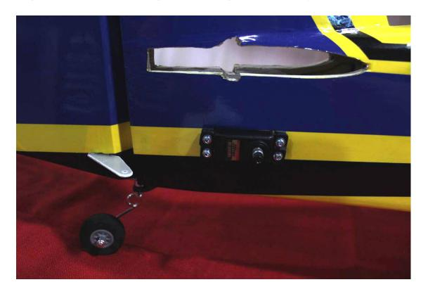
22. Install the rudder pushrod as shown. Use Loctite on the nuts.
