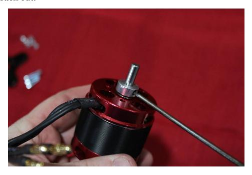
34. Next, secure the radial mount to the motor using the provided short Phillip's head machine screws. Again be sure to use a drop of blue Loctite on each screw.
