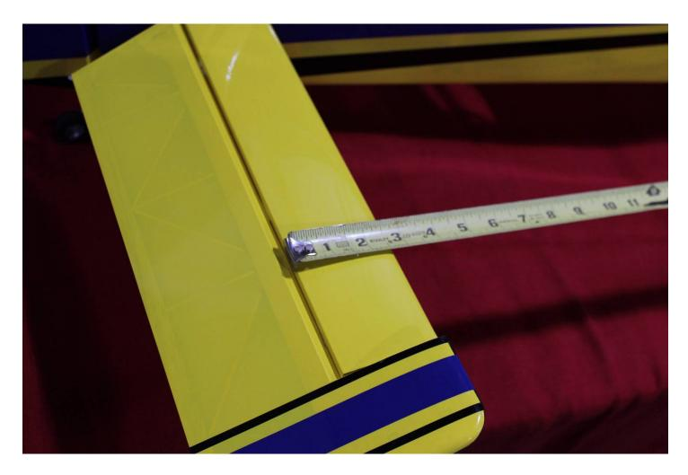
26. Once satisfied with the alignment, glue the horizontal stab in place by applying CA along the joint between the stab and fuse. Make sure to apply CA to the top and bottom
