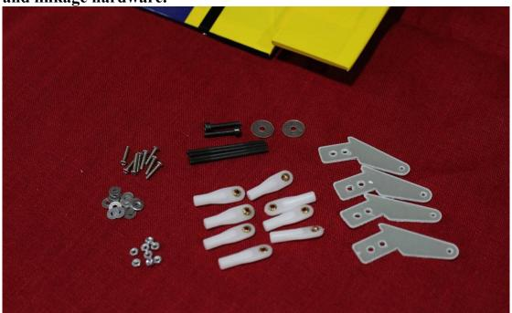
2. Use a soldering iron or sharp hobby blade to remove the covering over the slots for the aileron and flap horns. Make sure you are doing this on the bottom of the wing! Test-fit the horns – NO GLUE YET.
