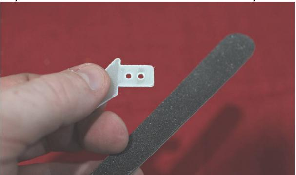
4. Apply 30 minute epoxy to the slot in the aileron and the scuffed potion of the control horn that will insert into the aileron or flap. Use a zip tie or toothpick to ensure the slot is completely filled with epoxy. Install the aileron horn into the aileron slot and wipe away any excess epoxy with a paper towel or cloth soaked with denatured alcohol. Allow to dry.
