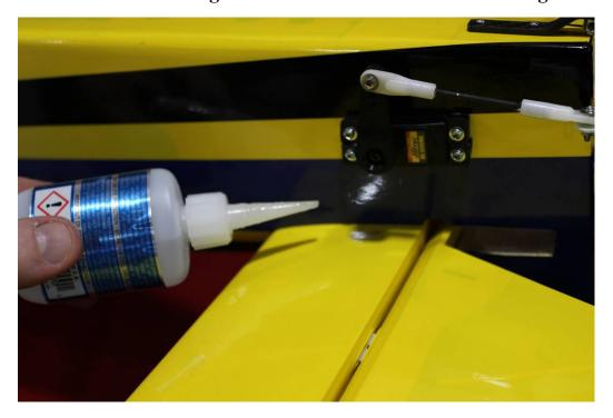
27. Align the elevator perfectly, flex it to make sure it moves easily 45 degrees up and 45 degrees down, and glue with several drops of thin CA per hinge.
