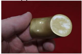
Use 30min epoxy or 'goop' or 'welder' type adhesive to glue the stacks to the cowl.
