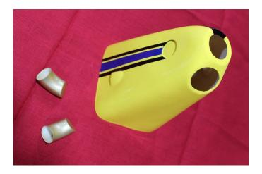
Scuff the mounting surface of the stack as shown, and the mounting area on the cowl, with sandpaper.
