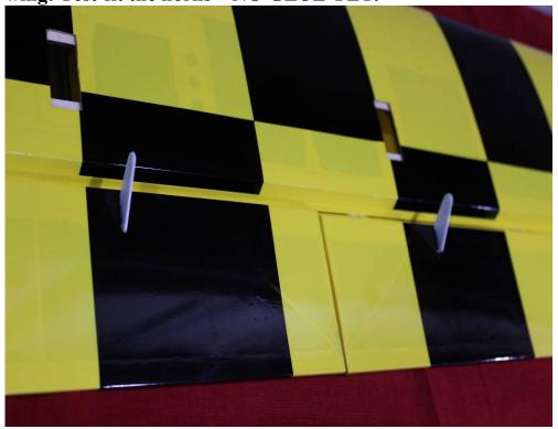
3. Once you are satisfied with the fit of the horns, remove them. Use sandpaper to scuff the portion of the horn that will be inserted into the aileron or flap.
