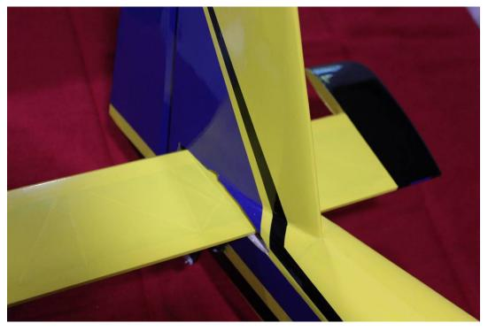
24. Slide the horizontal stabilizer into the slot, slide the elevator into position on its hinges, but do not glue yet.
