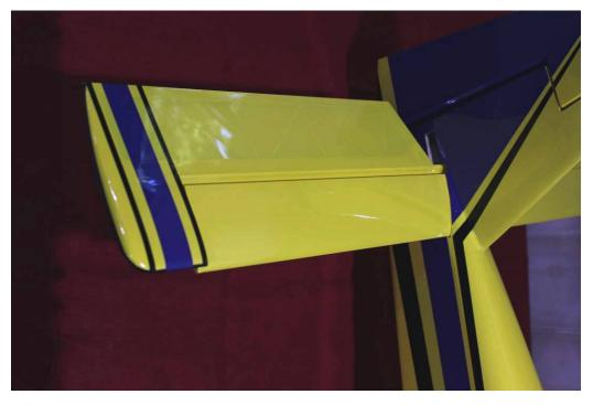
25. Install the carbon fiber wing tube into the fuselage and use a tape measure as shown to make sure the horizontal stabilizer is straight to the fuselage and perfectly
