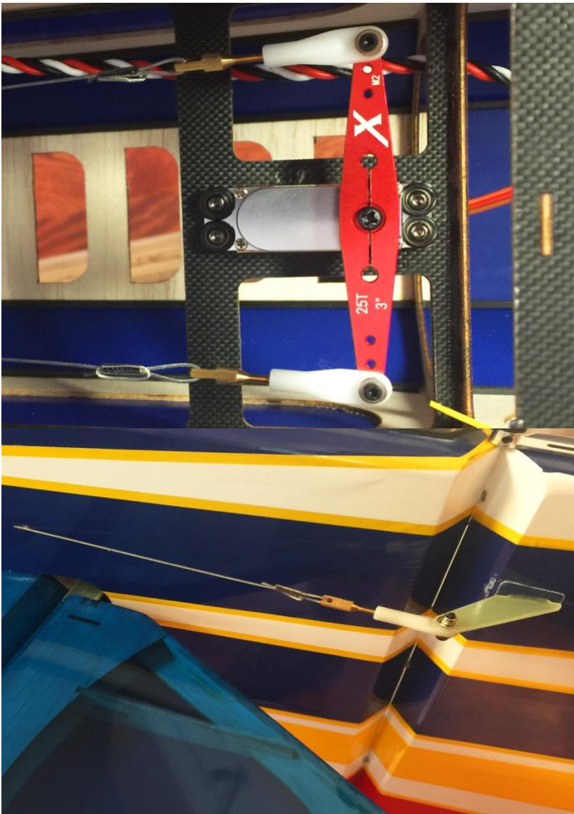
12. Install the tailwheel assembly as shown.
