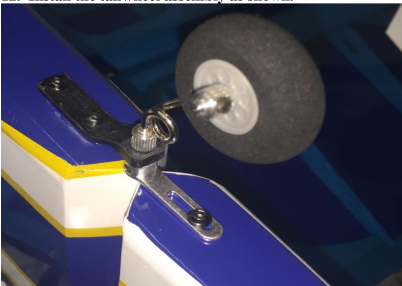
12. Install the tailwheel assembly as shown.
