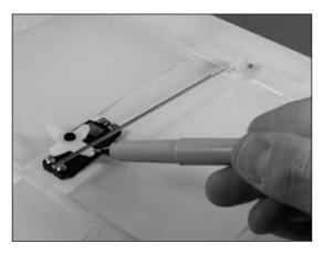
*Hint:* Use painter's tape to tape the aileron to the wing tip. This will hold the aileron in the centered position while you prepare the pushrod wire.
