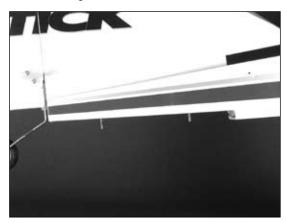
• 2. Attach the stabilizer using two 3mm washers and two 3mm locknuts. Do not tighten the locknuts all the way until after the wing is installed and you check the alignment.
