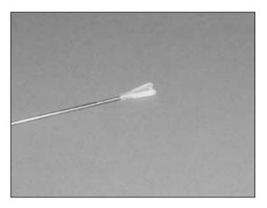
Q 4. Attach the clevis to the control horn. Plug the aileron servo into the receiver and turn on the radio. Center the aileron servo electronically. Use a felt-tipped pen to mark the pushrod wire where it crosses the servo horn.
