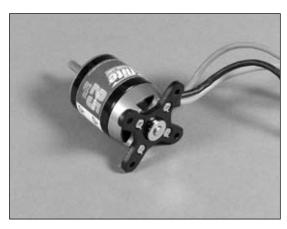
2. Place the four 4-40 blind nuts on the inside of the firewall in the locations for your particular motor. Attach the Outrunner motor to the front of the firewall using four 4-40 x 3/8" socket head screws.
