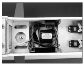
O 3. Thread a clevis onto the 22 1/2" (572mm) pushrod wire for the rudder. Slide the pushrod into the pushrod tube and attach the clevis to the rudder control horn.
