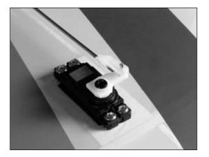
**Note**: Use side cutters to trim down the excess pushrod wire and remove the extra arms from the servo horn.
