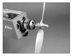
**Note**: It is very important that you check to be sure the propeller is balanced before installing onto the shaft. An unbalanced propeller will cause performance issues.
