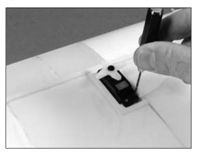
O 2. Secure the servo using the hardware that was provided with the servo.
