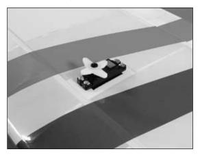
3. Attach a clevis onto the  $5^{5}/8^{11}$  (143mm) pushrod wire. Remove the backplate from the control horn and attach the clevis to the horn.
