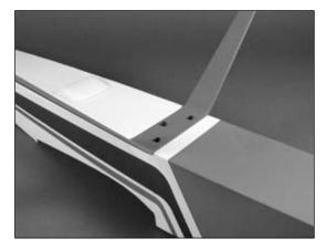
**Note**: The landing gear will only fit one direction for the holes to line up properly.
