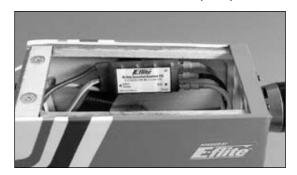
**Note**: It is wise to place a current meter in line with the ESC to check for current draw during full servo operation. Please see page 29 for further details.
