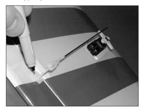
○ 5. Use a 5/32" (2mm) drill to drill the two holes for the control horn mounting screws. Use the backplate and two 2mm x 12mm screws to attach the control horn to the aileron.
