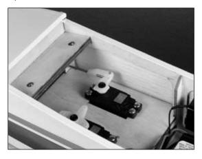
**Note**: Use side cutters to trim down the excess pushrod wire and remove the extra arms from the serve horn.
