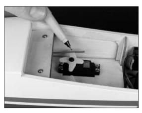
○ 5. Bend the pushrod wire at the mark made in the previous step. Enlarge the hole in the servo arm using a 5/64" (2mm) drill bit. Secure the pushrod wire to the servo horn using a pushrod connector.
