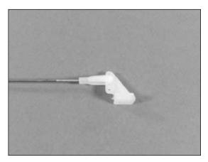
• 4. Position the control horn onto the aileron. Match the fore-aft position of the horn to the one preinstalled. The pushrod wire will be parallel to the wing ribs. Mark the location for the screws using a felt-tipped pen.
