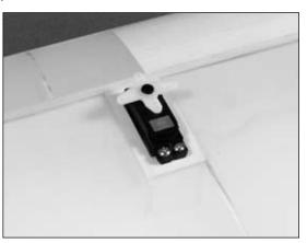
O 3. Attach the clevis to the 5<sup>5</sup>/<sub>8</sub>" (143mm) pushrod wire. Thread the clevis onto the pushrod wire at least 12 turns.
