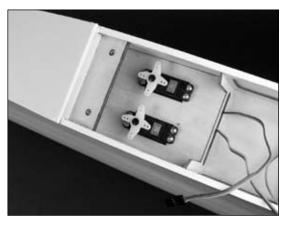
• 2. Plug in the servos and ESC into the receiver. Mount the receiver to the side of the fuselage using hook and loop material. Route the antenna wire through the bottom of the fuselage to the rear.
