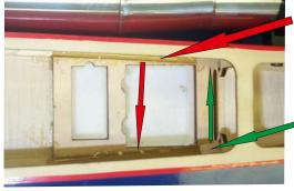
Before installing the servos we recommend you bead 5 min epoxy on either side of the servo tray to ensure security and to aid the fixture of the throttle servo.
