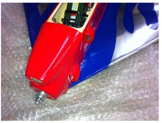
With a sanding drum cut hole as per picture in back of canopy to allow air flow out of the airframe.
