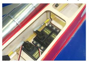
Insert the 2mm nut on the end of the thread followed by the 2mm metal clevis. This needs to be repeated at the other end. All this is done in conjunction with the positioning of the horn over the hinge point of the control surface and at the correct angle as per pic below. Secure the control horns in place with the supplied bolts and nuts.
