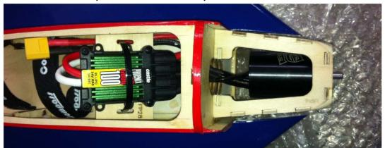
Install ESC to tray and secure in place with a tie-wrap
