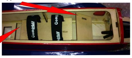
Install the battery tray with epoxy as per the picture. We recommend installing the velcro straps before the tray is installed.
