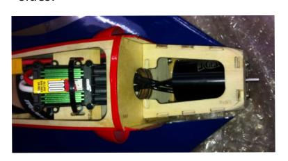
When happy install the cowling with the 4 supplied screws.
