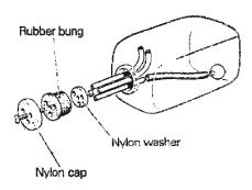
The two bent vent tubes should be pointing upwards in the bottle and the tank can be assembled with either the narrow or wide side of the bottle uppermost to suit the shape and size of your fuselage.
