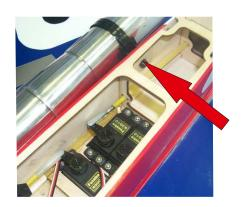
Using a silicone joiner which is available from Weston UK join the tuned pipe to the manifold. Mark the position of the tuned pipe on the mounting plate at the rear giving yourself enough room to insert the bolt for the canopy. When happy bolt the airframe clamp available from Weston UK to the fuselage and tie-wrap the tuned pipe to the clamp.
