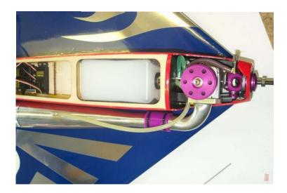
Install the manifold and the tuned pipe which are available from Weston UK as shown.
