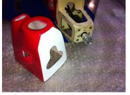
Mark up positions of side cheek cooling ducts and cut holes as required ensuring you key the surface of the area where the cooling ducts will be fitted. Ensure the cooling ducts are not to low to ensure clearance of the wing. We recommend cutting an air out hole at the bottom of the cowling as per pic.
