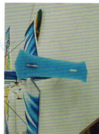
Install epp speed brake on tail using foam glue.
