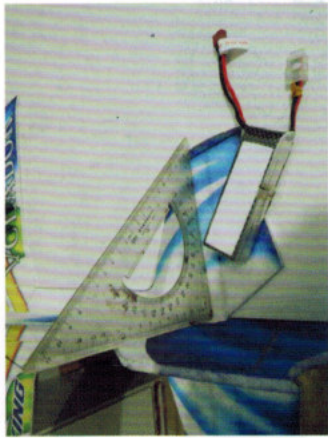
Must check whole fuselage to ensure fuselage orthogonality before glue dry.
