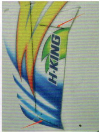
Install the carbon strips on aileron using foam glue.
