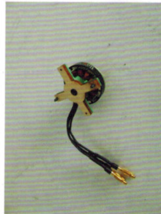
Assemble motor on the metal cross using screws. Then install motor on motor mount with tapping screws (we can use servo's screws).
