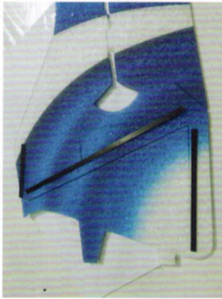
Install the 3 pcs carbon strips on rudder using foam glue.
