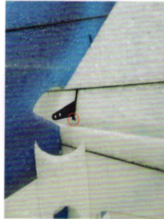
Cut the hinge when install hinge on elevator.
