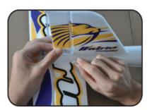
4. Install and fix the main wing, Push the wing rod into the wing as shown. Fix the main wing panel to the fuselage. Use a tool to fix and install the main wing onto the fuselage.
