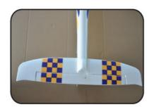
3. Use a tool to fix and install the stabilizer as shown. Glue the stabilizer on the fuselage. Then connect the control rod.
