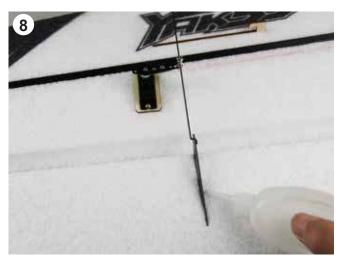
Glue the control horn as shown. Attach the "Z-bend" pushrod to the control horn and lock it with the pushrod connector.
