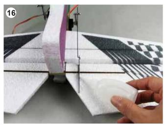
Install "Z-bend" pushrod to the control horn and lock it with the push rod connector. Then apply CA glue to the control horn.
