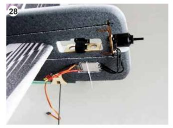
Install the ESC onto the fuselage and secure it with a zip tie.
