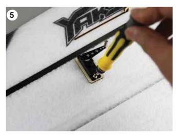
We will make the right wing first. Insert the aileron servo and servo mount to the pre-cut servo slot. Ensure those servo wires are properly organised during the installation.
