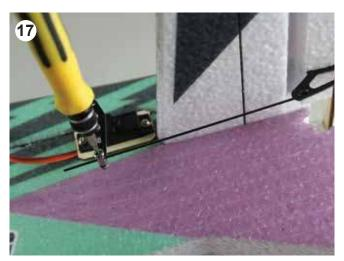
Tighten the grub screw and loctite it.
