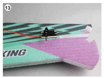
Install rudder servo with servo mount on the rear part of the fuselage as shown.
