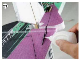
Apply CA glue to the rudder horn.
