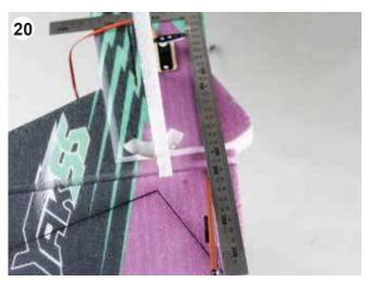
Use the same technique as shown above to prepare the control horn installation on the rudder.
