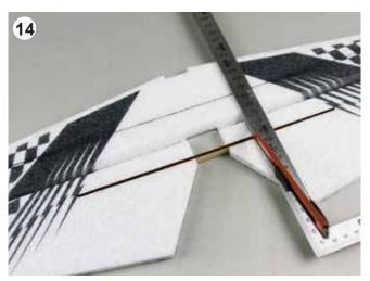
Cut a slot for the elevator control horn as shown .
