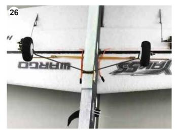
Install the landing gear on the gear mount.
