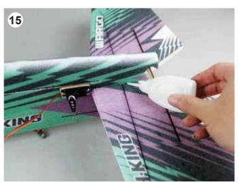
Trail fit the elevator onto the fuselage. Ensure it is straight and level to the fuselage and main wing. Then apply CA glue to the joint between the elevator and fuselage.
