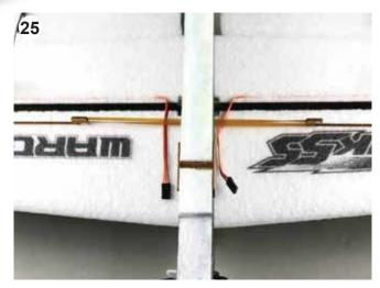
There are two ways to fix the wings onto the fuselage. 1. Connect the wings with two rubber bands as shown in picture #25. You can remove the wings during transportation and for easy storage.
