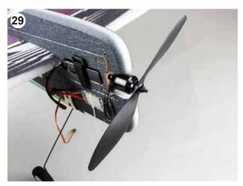
Secure the battery flight pack to the fuselage with the velcro band provided.
