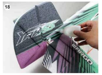
Install the vertical stabiliser to the fuselage. Please ensure that it's perpendicular to the horizontal stabiliser.
