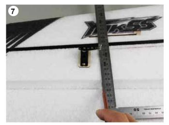
Cut a slot on the aileron strip which is perpendicular to the servo arm with a hobby knife as picture shown.
