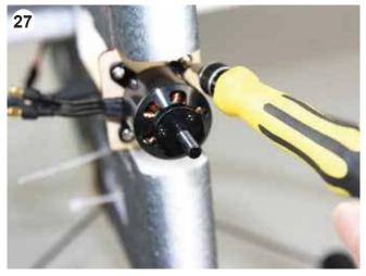
Install the brushless motor onto the motor mount and secure it with 4 tapping screws provided with the kit.
