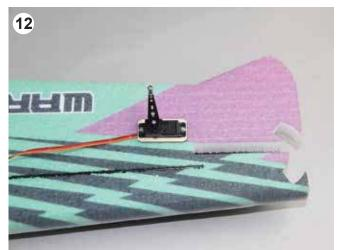
Install the elevator servo with the servo mount as shown.
