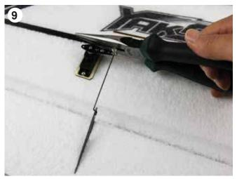
Trim the excess pushrod wire with a wire cutter. Then smooth the cut with a file.
