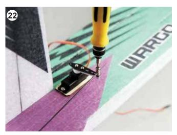
Install "Z-bend" pushrod as shown and lock it with the pushrod connector.
