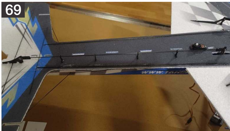
69. Above is the finished linkage setup with elevator centered and rod well fitted and glued in both the quick links with all the guides in place.
