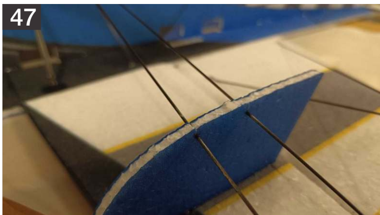
47. Make a small slot on bracing support using a sharp knife where it meets the rod. Make sure the carbon bracing is slid about a mm down into the slots.
