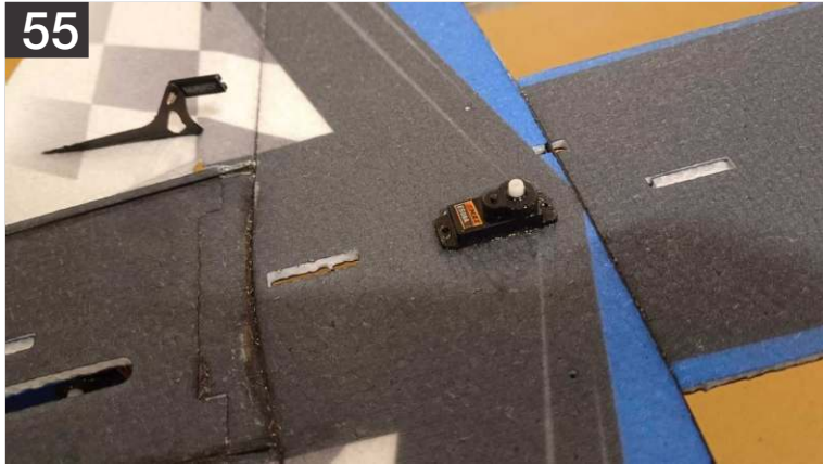
55. Time to install the servos, put the aileron servo in place and glue it.
