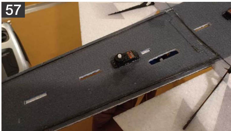
57. Glue the rudder servo in place.
