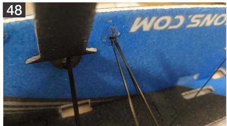
48. Shown above is how the wing bracing rods glued with the last fuselage bracing just behind the undercarriage, on the fuselage.
