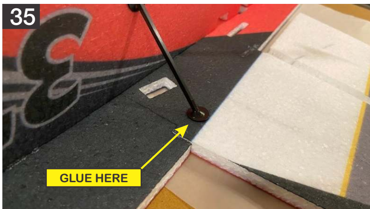
35. Put a drop of HV CA over the joints and spray everything together.
