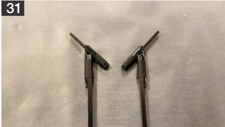
31. Optionally use a heat shrink tubing for better cosmetic finish.
