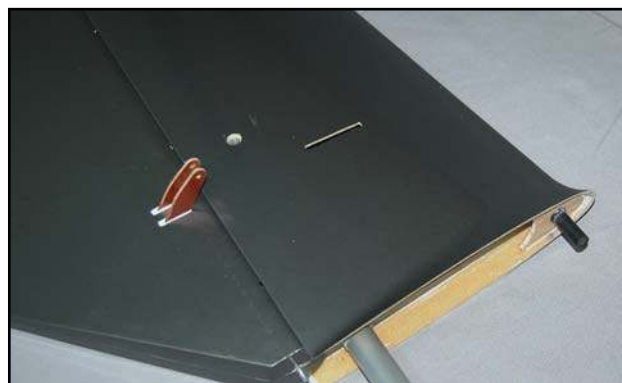
(above) Elevator horns, spar tubes, stab securing bolts, anti-rotation dowels and servo arm slots are all factory-finished.
