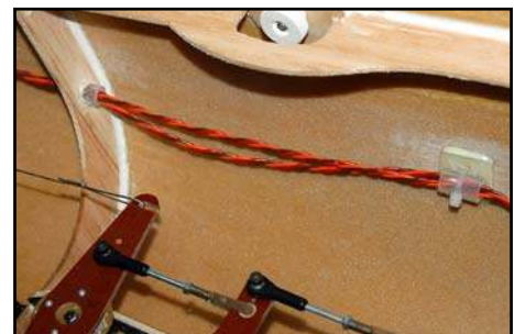
(below) Protect all wires and tubes where they pass thru' bulkheads, or near sharp composite parts, with a short length of silicone tube, and cable-tie firmly in position.
