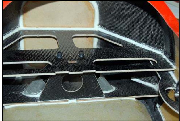
(above) The carbon legs are secured using the M6 x 20mm bolts and large washers.
