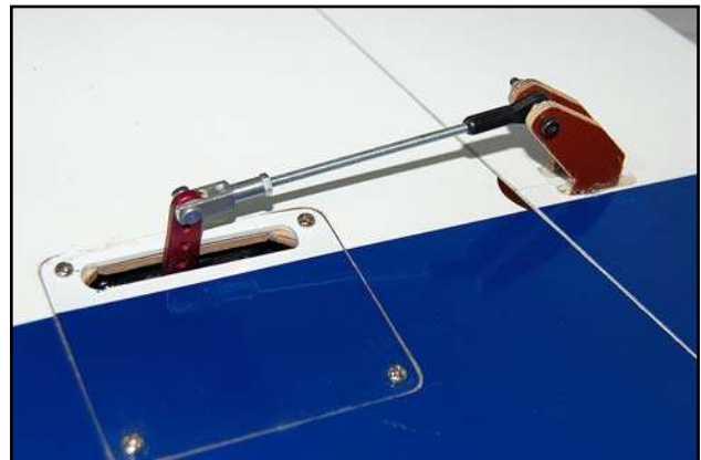
(below) Aileron linkages are assembled using the provided hardware. Outer servo hatch is secured with Ø 2.9 x 10mm screws. Mill the slots in the hatches to suit your metal servo arms.
