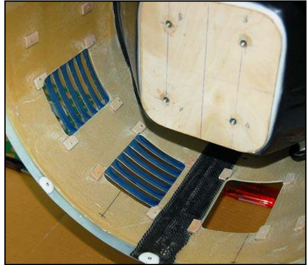
(above) Only the lower 4 louvres have cutouts, the top 4 louvres are just 'dummy' air vents, and should not be cut out.
