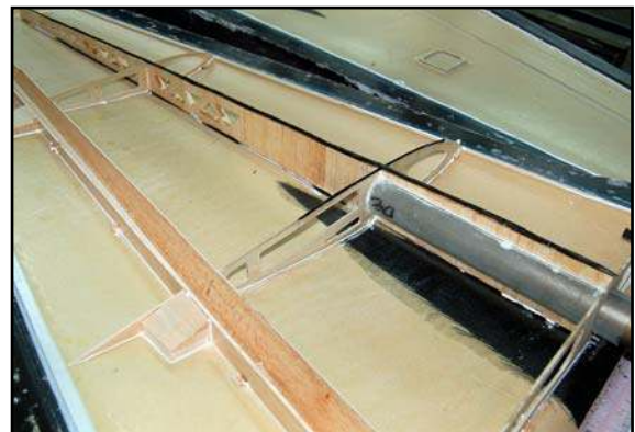
(above) The internal wing structure, showing the carbon roving and cloth reinforcement.
