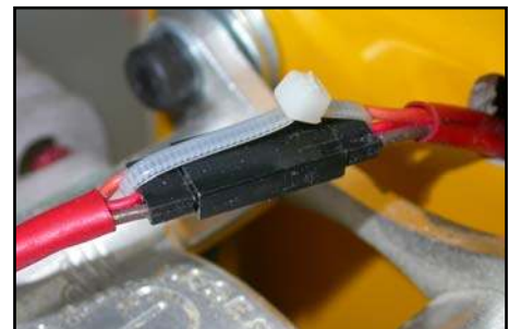
(below) Secure the connection between the motor pick-up and the ignition plug with heatshrink tube of a very small cable-tie.
