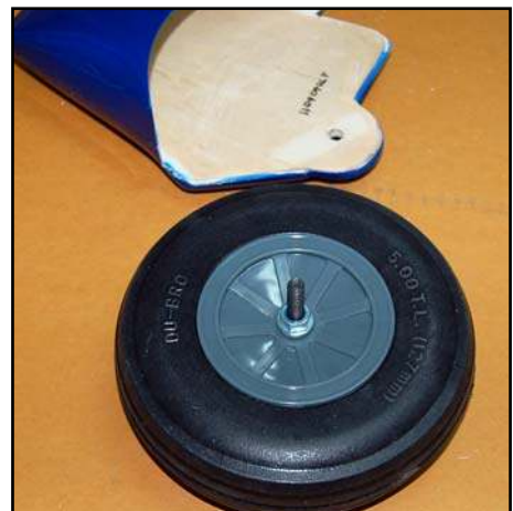
(left/below) Completed wheelpant with 5" Dubro wheels. The angle of the wheelpants to the legs is set with 2 small sheetmetal screws, thru' the wheelpant into the carbon leg.
