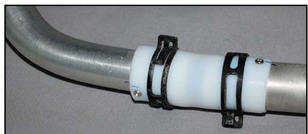
(below) 2 small screws thru' the Teflon joiners prevent the cans moving in flight.
