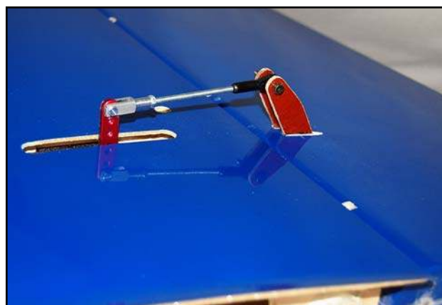
(below) Milled 3mm thick plywood doublers are included for both the JR8711/8811 and the Futaba S9152 servos. JR8811 and SWB 1.5" servo arm shown here.
