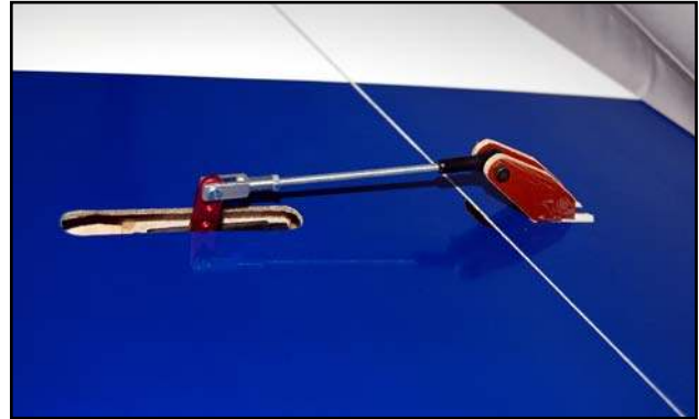
(above) Inner servo linkage shown using a single servo, installed in the rear of the phenolic mount. If using dual 'ganged' servos you will need to extend the servo arm slot forwards for clearance on the front servo arm.
