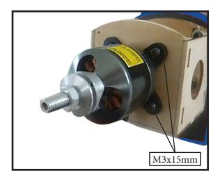
4) Locate the plywood battery tray to the fuselage. Tighten the screws using machine screws M3x15mm to secure the tray in position.
