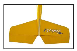
8) After the epoxy has fully cured, remove the masking tape or T-pins used to hold the stabilizer in place. Carefully inspect the glue joints. Use more epoxy to fill in any gaps that may exist that were not filled previously and clean up the excess using a paper towel and rubbing alcohol.
