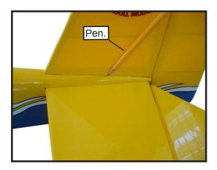
2) Using a modeling knife, remove the covering from over the precut hinge slot cut into the lower rear portion of the fuselage.
