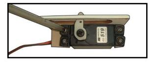
7) Apply 1-2 drops of thin C/A to each of the mounting tabs. Allow the C/A to cure without using accelerator.
