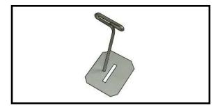
2) Remove each hinge from the wing panel and aileron and place a T-pin in the center of each hinge. Slide each hinge into the aileron until the T-pin is snug against the aileron. This will help ensure an equal amount of hinge is on either side of the hinge line when the aileron is mounted to the wing panel.
