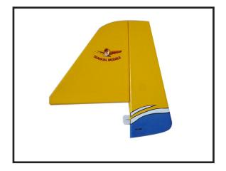
1) While holding the vertical stabilizer firmly in place, use a pen and draw a line on each side of the vertical stabilizer where it meets the top of the fuselage.
