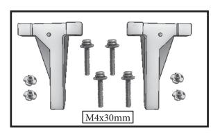
2) Use four 4x30mm head bolts and four 4mm washers to attach the engine mount rails to the firewall. Tighten the screws . Make sure to use threadlock on the screws to help prevent them from vibrating loose.
