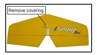
When cutting through the covering to remove it, cut with only enough pressure to only cut through the covering itself. Cutting into the balsa structure may weaken it.
